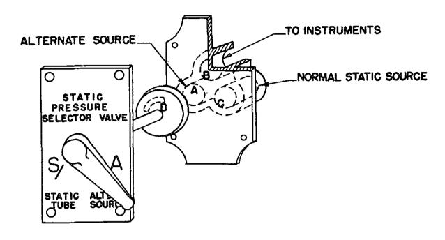
STATIC VALVE - ALTERNATE POSITION WITH HANDLE IN POSITION "A" CHANNEL "D" CONNECTS "A" (ALTERNATE STATIC SOURCE) TO "B" (INSTRUMENTS).
