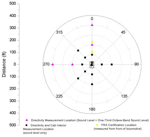
**Figure 2. Plan View of Measurement Locations**
