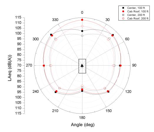
Figure 3. Center-Installed vs. Cab Roof Installed Sound Levels
