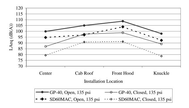
Figure 4. Locomotive Cab Interior Noise Levels
