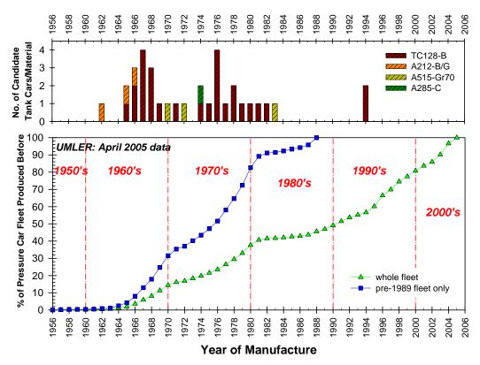
Figure 2: Cumulative Distribution of Pressure Tank Car Fleet and Tank Cars Used for Testing
