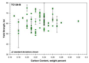
Figure 7: Poor correlation between carbon content and yield strength for TC128-B steel.
