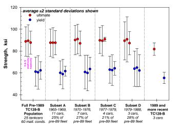
Figure 3: Strength properties of the tank car fleet.
