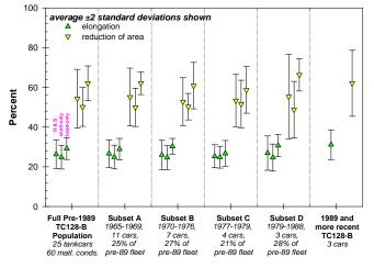
Figure 4: Ductility properties of the tank car fleet.
