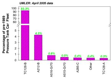
Material Used in Tank Car Fabrication
