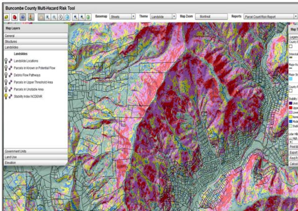
*The tool can highlight areas that might be affected by a landslide debris flow and other natural hazards.*
