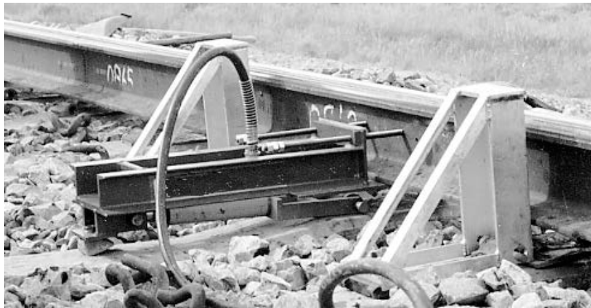
Figure B-2. STPT Equipment for Concrete Ties
