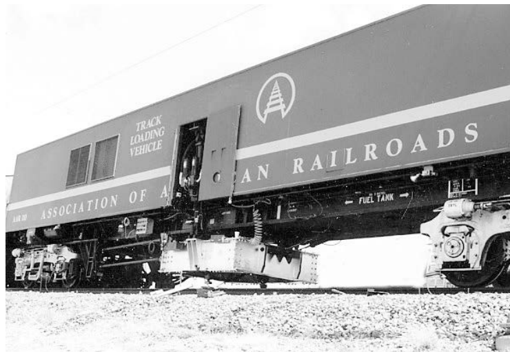
Figure B-12. TLV Based Rail Uplift Measurements
