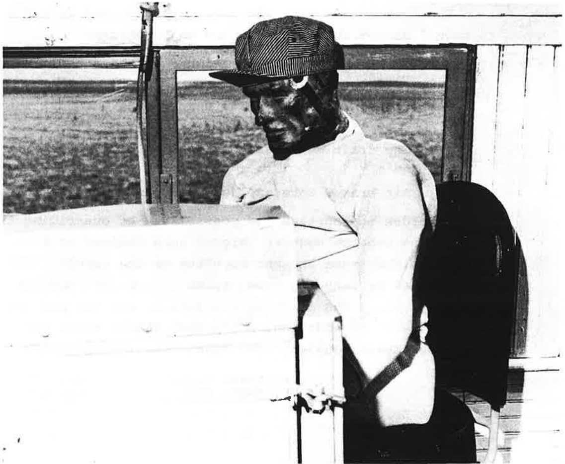
FIGURE 19. ANTHROPOMORPHIC 95TH PERCENTILE MALE DUMMY PLACED IN THE LOCOMOTIVE OPERATORS SEATING POSITION.
