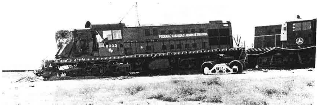
FIGURE 47. POST-TEST IMPACTING LOCOMOTIVE SOUTH SIDE - TEST 9.
