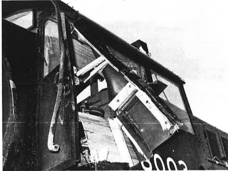
FIGURE 49. POST-TEST IMPACTING LOCOMOTIVE CAB - TEST 9.
