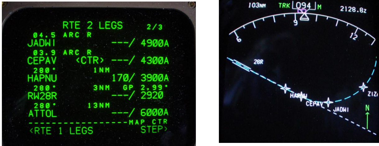
Figure 10. Boise runway 28 Right, final segment of the Emmett transition on the CDU (left) and ND (right).
