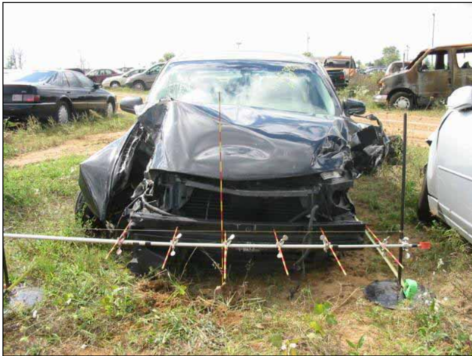
Figure 21. Case 2003-12-162 Showing Fire Hydrant Damage on Vehicle's Right
