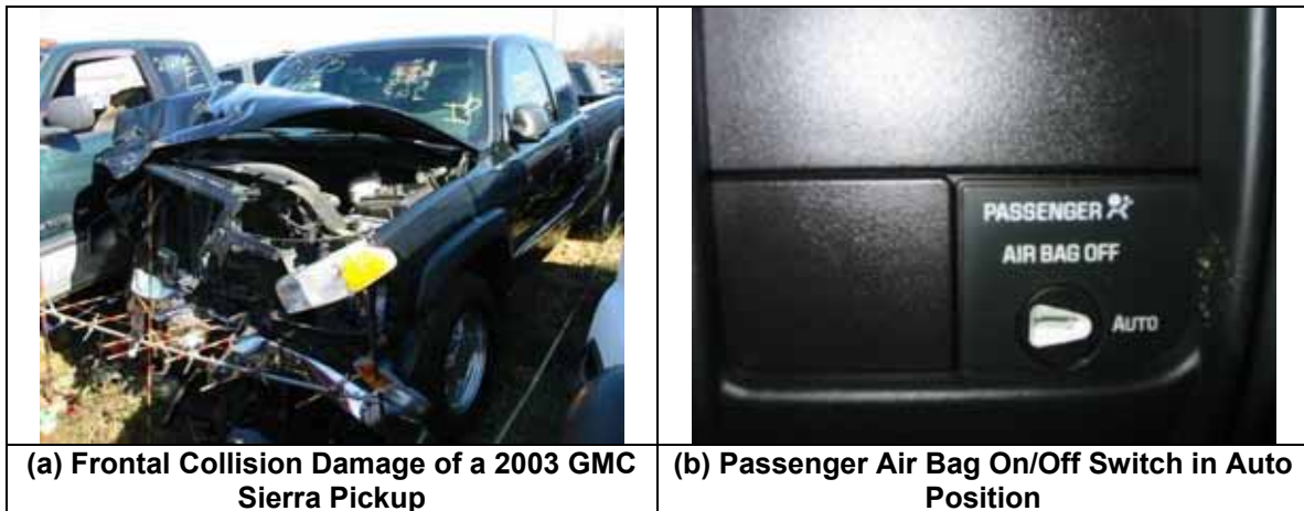
Figure 23. Frontal Crash in Which Driver Air Bag Deployed, But Passenger Air Bag Did Not in the Presence of an Adult Right-Front Passenger (NASS 2003-09-224)
