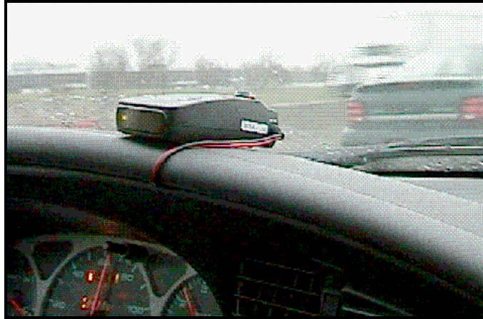
Figure 2. Gary-Chicago-Milwaukee Corridor In-Vehicle Warning Device [3]
