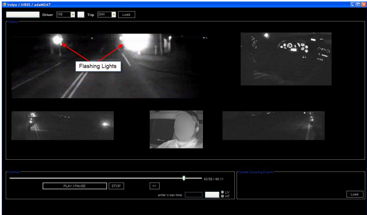
Figure 9. Snapshot of an Event at a Highway-Rail Crossing Equipped with Flashing Lights
