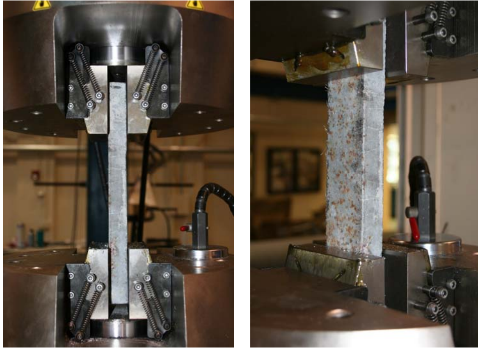
Figure 29. Photo. Two photos of the direct tensile testing of a UHPC prism.
