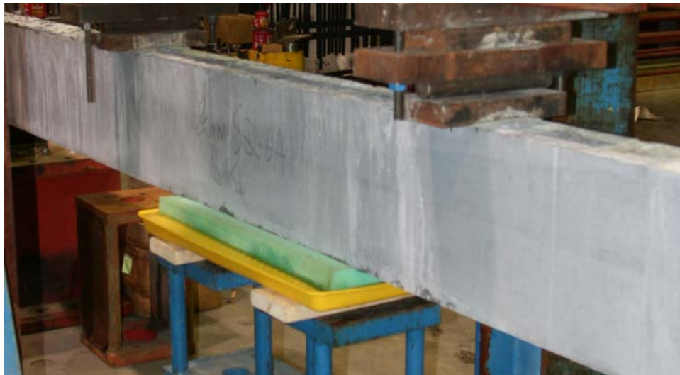
Figure 6. Photo. Salt water solution application system.
