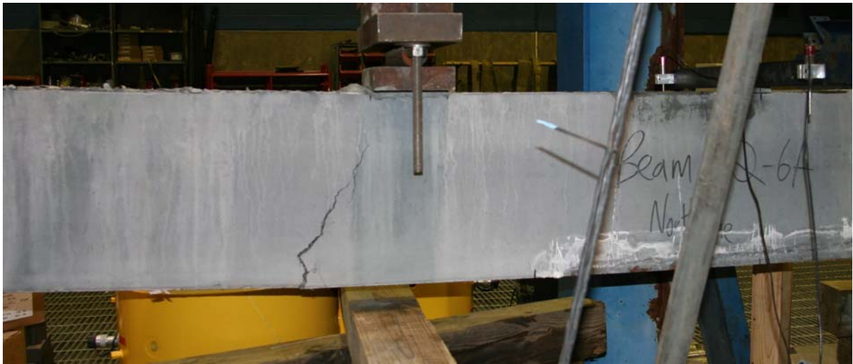
Figure 20. Photo. Failure crack east of east load point.
