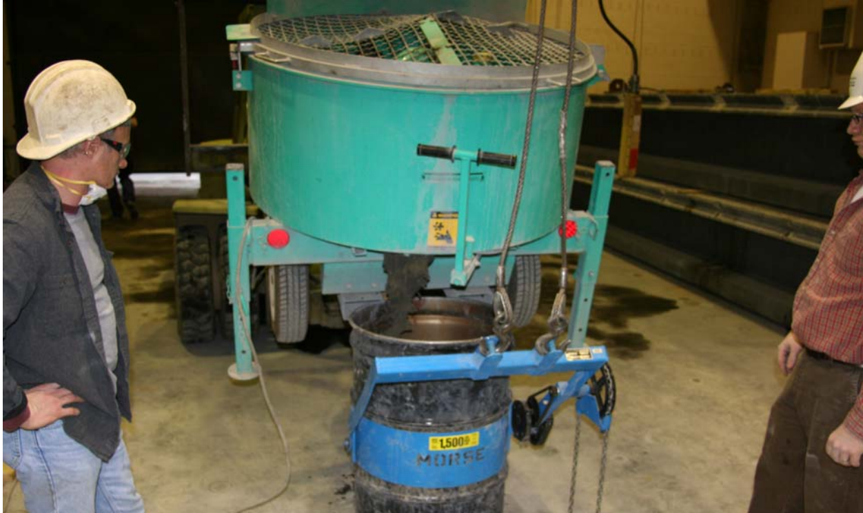
Figure 1. Photo. Discharge of UHPC holding barrel.
