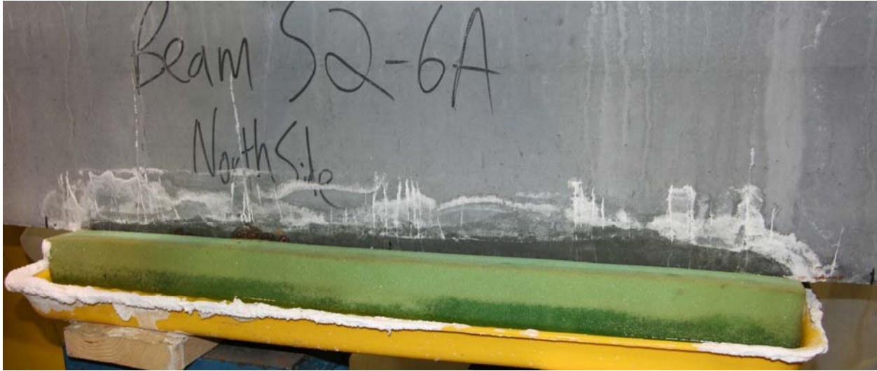
Figure 13. Photo. North face of beam near midspan immediately after the conclusion of the third phase of cyclic testing.
