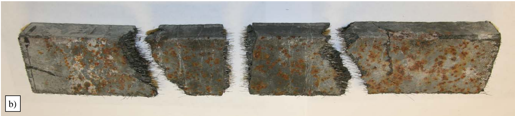
Figure 33. Photo. Failed UHPC tensile prism after a) second test and b) third test.
