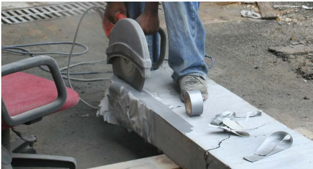
Figure 28. Photo. Extraction of a prismatic specimen from beam tensile face.
