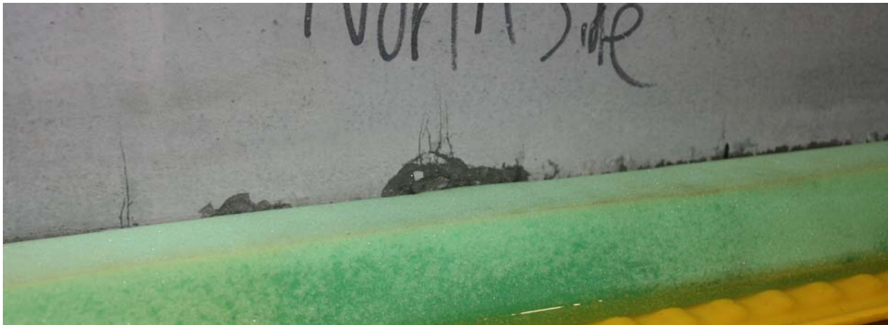
Figure 12. Photo. North face of beam near midspan one hour after the initiation of the third phase of cyclic testing.
