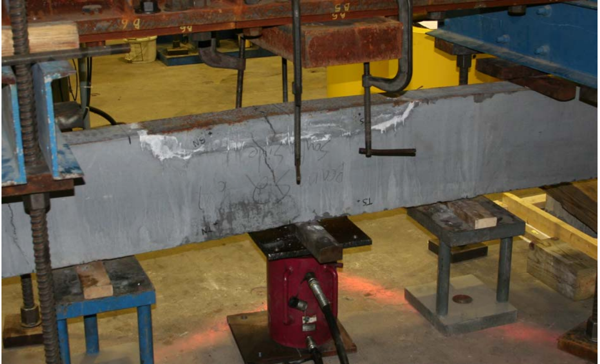
Figure 23. Photo. Beam failure near midspan after second subsequent flexural loading.
