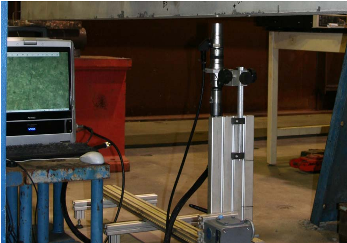
Figure 7. Photo. Crack assessment microscope and linear traverse system.
