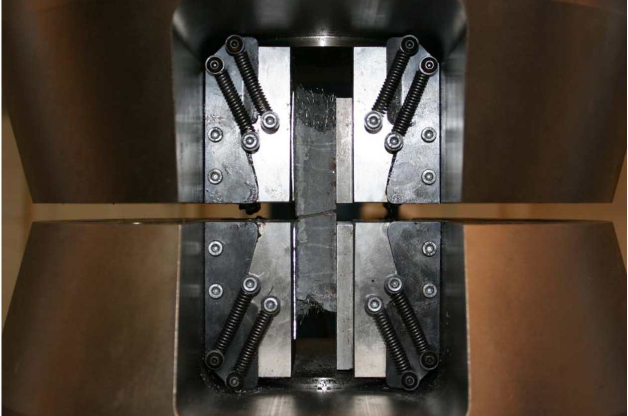
Figure 32. Photo. Third direct tensile test of a UHPC prism.
