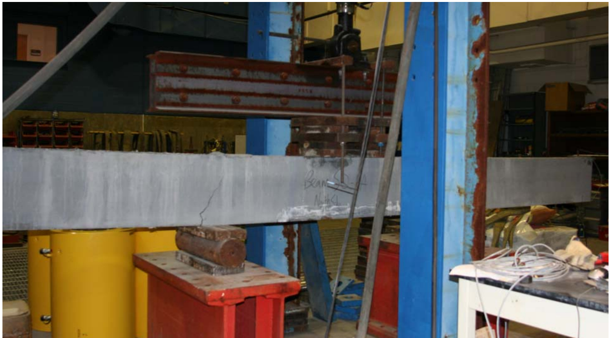
Figure 21. Photo. Test setup for first subsequent flexural loading.
