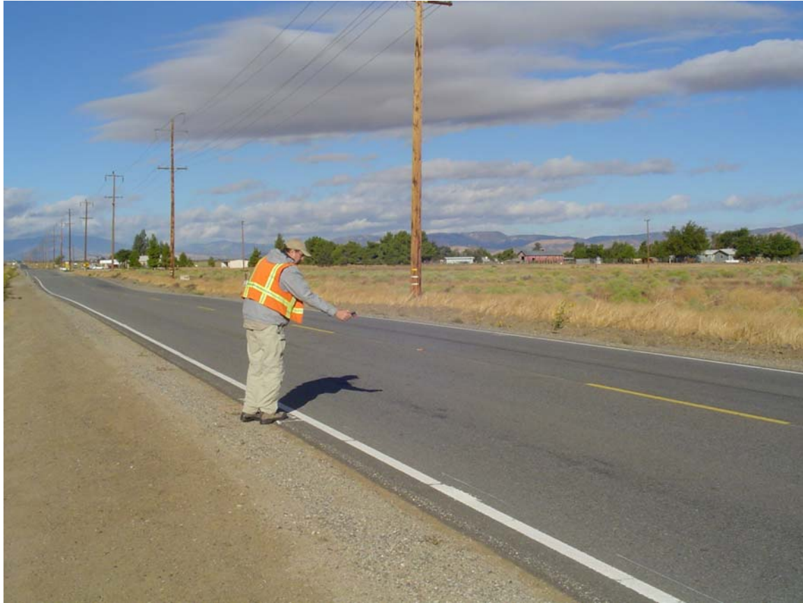
Figure B-5. Infrared temperature gun (also seen in Figure B-2).
