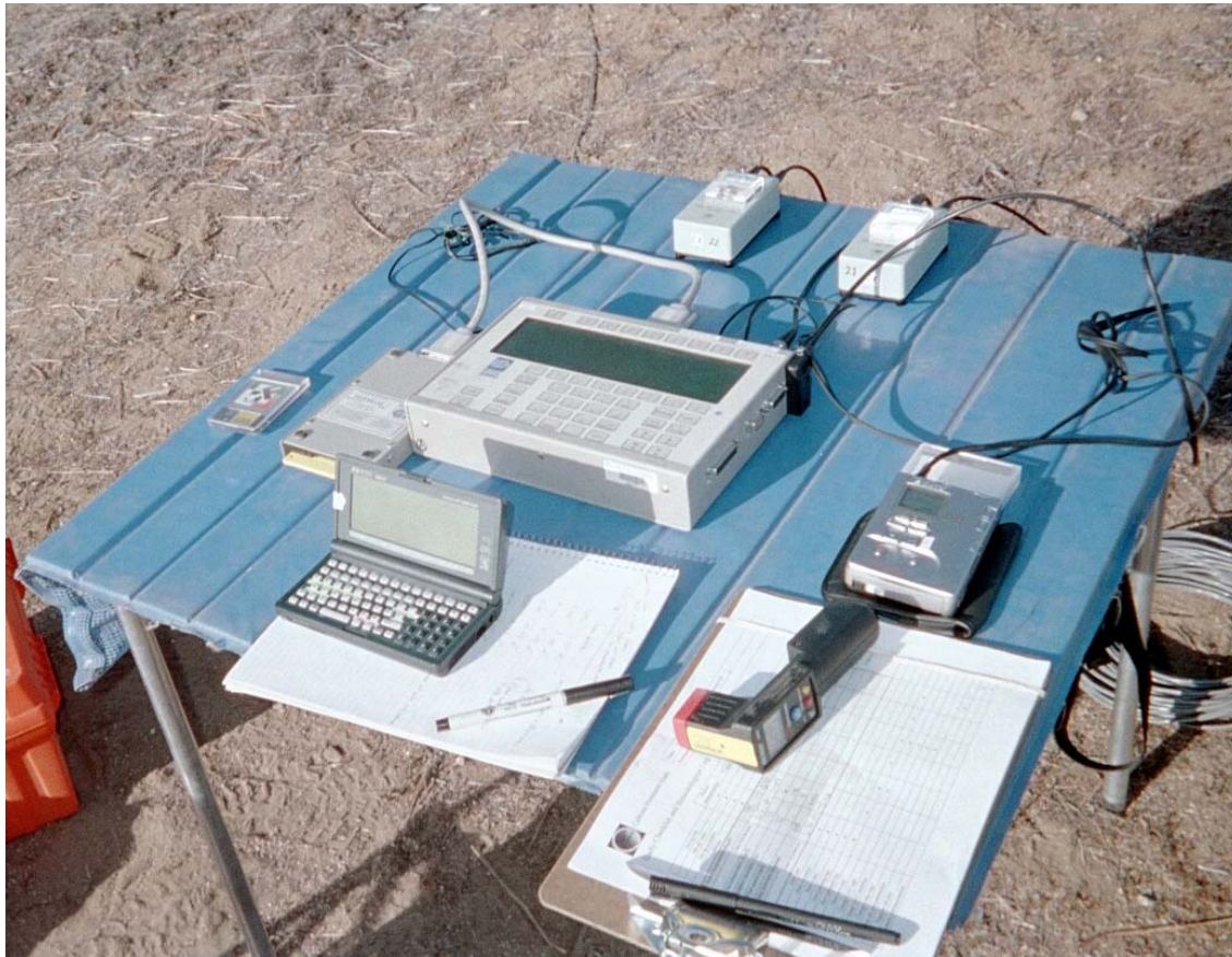
Figure B-2. Deployed spectrum analyzers (LDL Model 2900 2-Channel Spectrum Analyzers).
