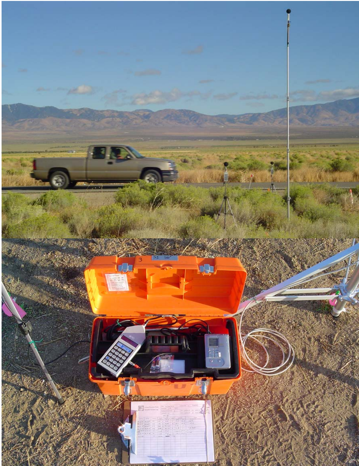
Figure B-1. Deployed sound level meters (LDL Model 820 Sound Level Meters) and DAT recorder (Sony Model TCD-D100 Digital Audio Tape (DAT) Recorder).
