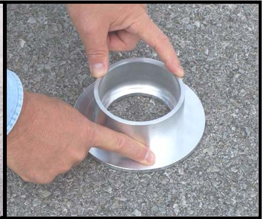
Fig. 9 – Pavement attachment fixture.
