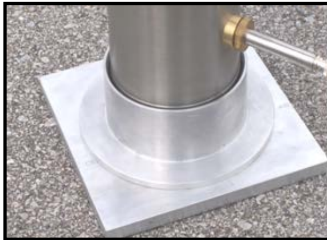
Fig. 10 – Measuring the reference absorption using a 10 mm thick plate.
