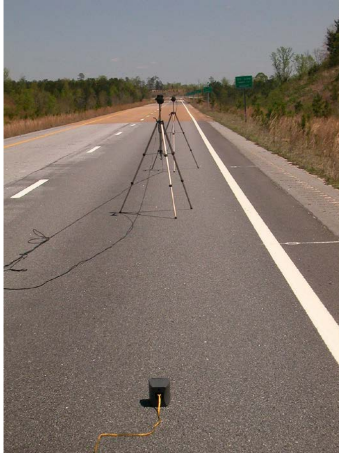
Fig. 5 - Instrumentation set-up for tire noise sound propagation measurements.
