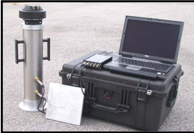
Fig. 8 – Sound absorption measurement system.
