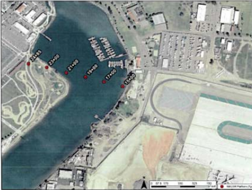
Figure 1 MALSR Environment off SAN Runway 9
