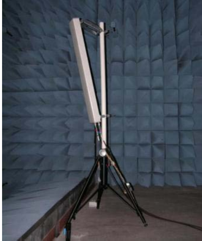
Figure 3. LightSquared Argus LTE Antenna
