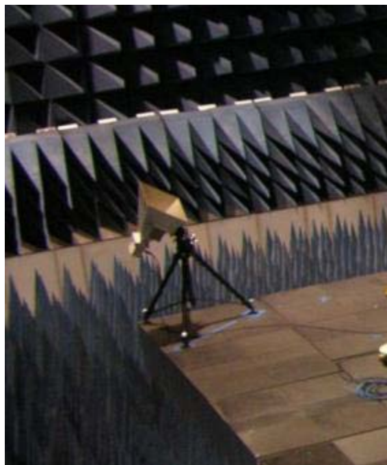
Figure 5. Mapping Receive Antenna at the ARL Reference Point
