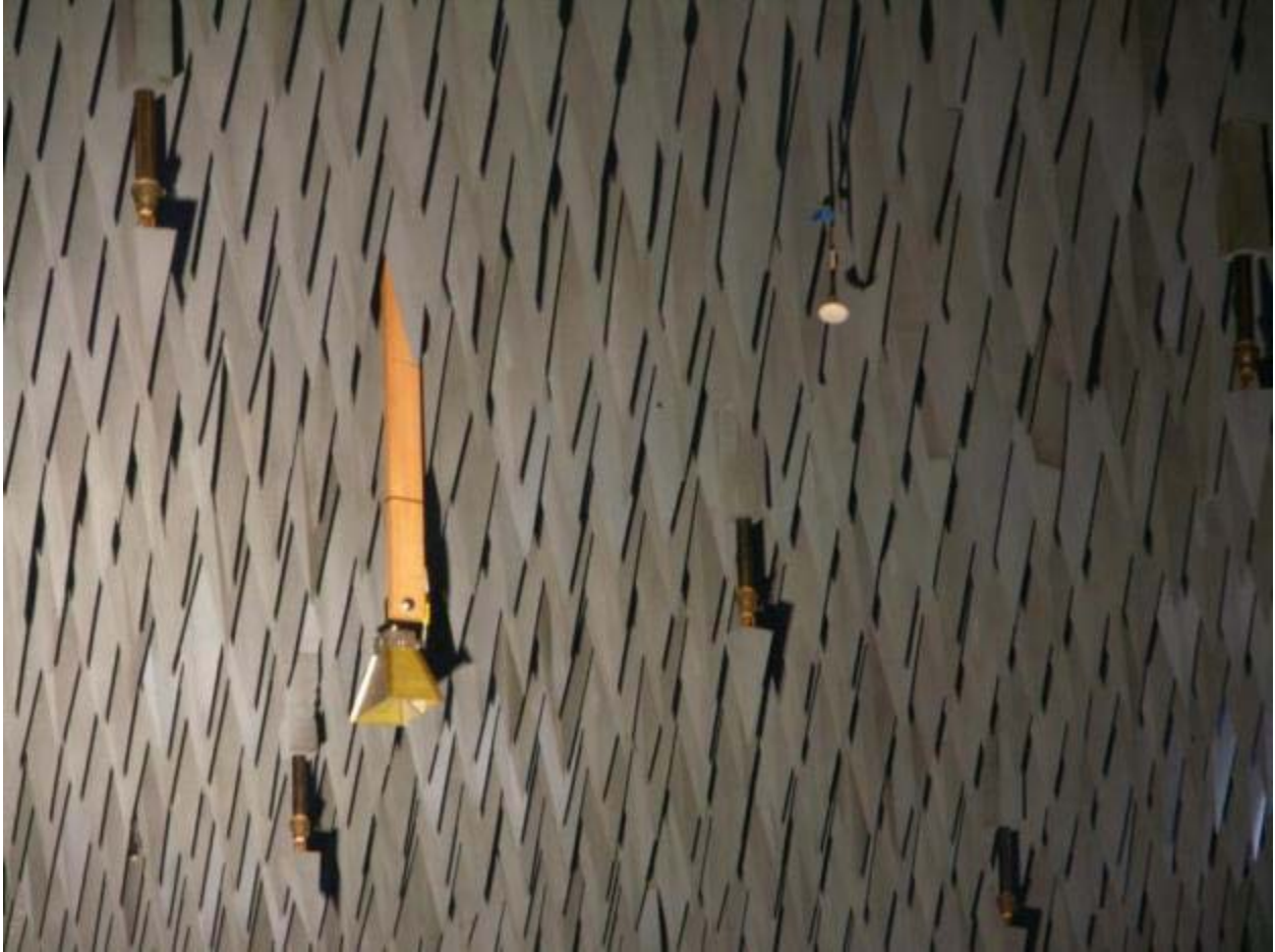
Figure 4. LightSquared Handset Surrogate Antenna (double ridge horn) and the GPS Broadcast Antenna
