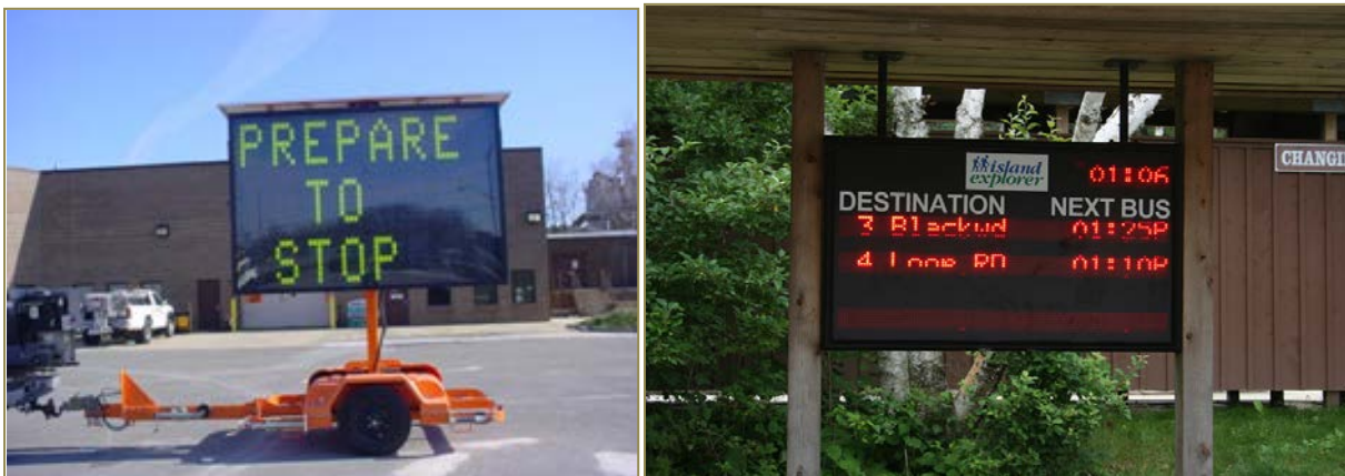
FIGURE 1 Dynamic message signs can be either portable, for use in multiple locations, or permanent fixtures at a specific location.
