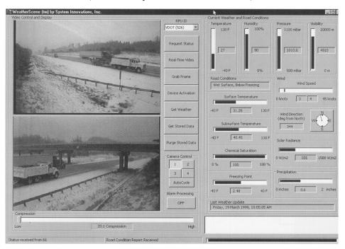
Figure 3-31. Weather imagery and data display (Picture courtesy of System Innovations, Fredericksburg, VA).
