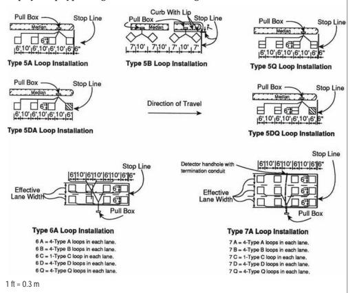
Figure 4-12. Caltrans standard sequential inductive-loop configurations.
