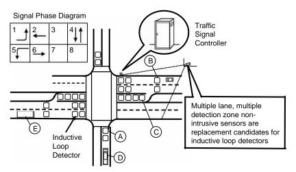
Figure 3-2. Isolated intersection control. The letters represent data sources that influence signal timing as explained in the text.
