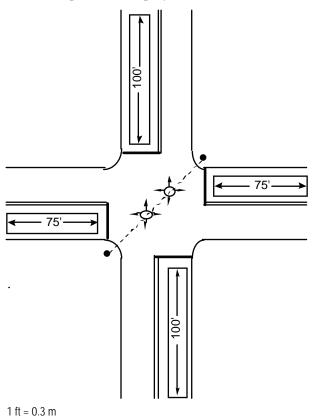
Figure 4-4. Intersection configured for loop occupancy control.
