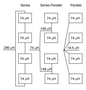
Figure 2-8. Four 6- x 6-ft (1.8- x 1.8-m) three-turn loops connected in series, parallel, and series-parallel.
