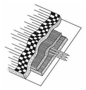
Figure 2-24. Five-layer temporary open loop detector configuration.
