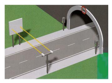
Figure 3-29. Overheight sensor configuration (Picture courtesy of MBB SensTech, Munich, Germany).
