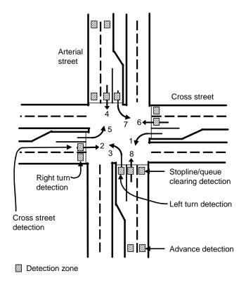
Figure 3-4. Placement of sensors for fully actuated intersection control. The numbers represent a four-phase signal sequence consisting of traffic movements 1 and 5, 2 and 6, 4 and 8, and 3 and 7.
