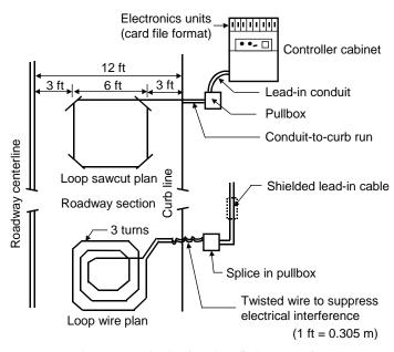
Figure 1-4. Inductive-loop installation example.
