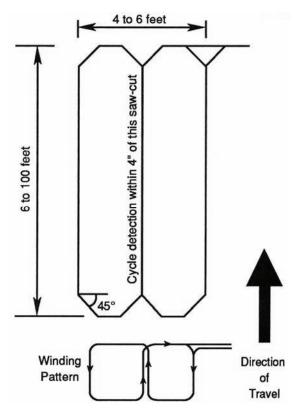
Figure 4-23. Quadrupole loop configuration.
