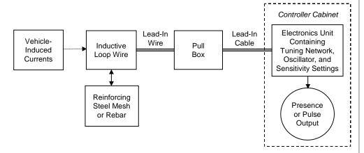
Figure 2-1. Inductive-loop detector system (notional).
