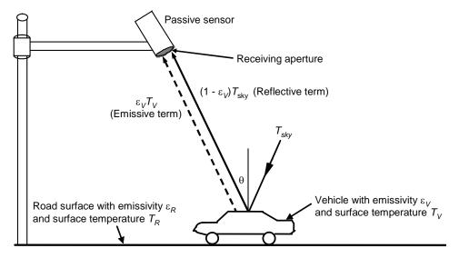
Figure 2-67. Emission and reflection of energy by vehicle and road surface.
