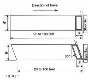
Figure 4-27. Long loop with powerhead.
