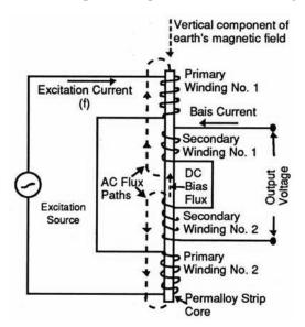
Figure 2-43. Magnetometer sensor electrical circuit (notional).
