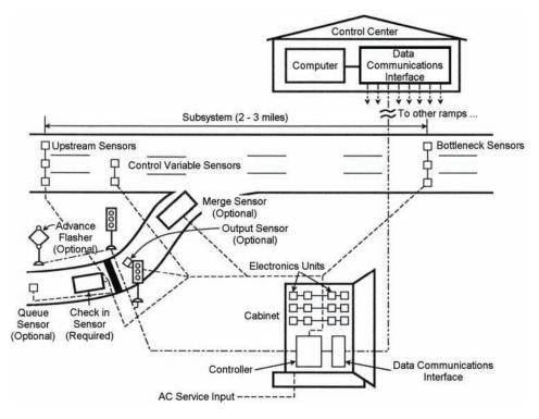
Figure 3-10. Conceptual coordinated traffic responsive ramp control system.
