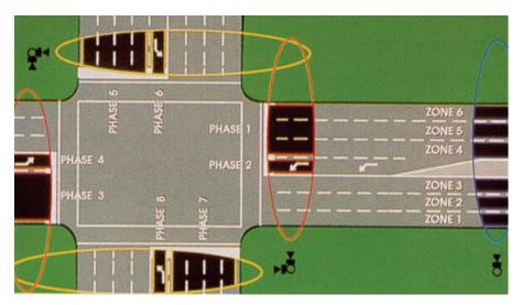
Figure 1-8. Mounting of presence-detecting microwave radar sensors for multilane vehicle detection and signal actuation at an intersection (Picture courtesy of EIS, Toronto, Canada).
