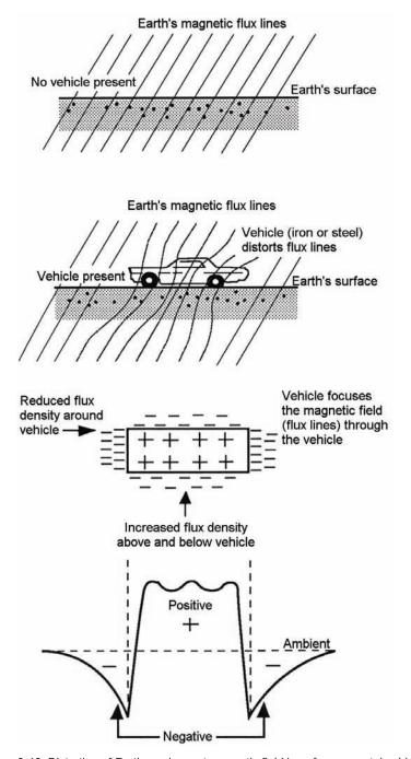
Figure 2-42. Distortion of Earth's quiescent magnetic field by a ferrous metal vehicle.
