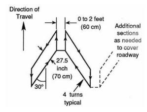
Figure 4-26. Chevron-loop configuration.
