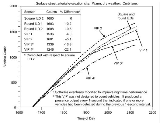
Figure 2-53. Vehicle count comparison from four VIPs and inductive-loop detectors (source: L.A. Klein and M.R. Kelley, *Detection Technology for IVHS: Final Report*, Report No. FHWA-RD-95-100 (USDOT, FHWA, Washington, D.C.,1995)).
