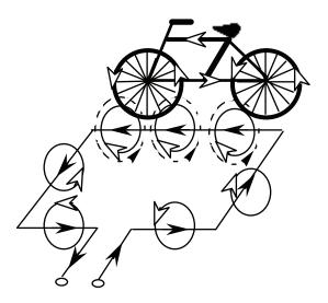
Figure 2-9. Bicycle detection showing induced eddy currents. The black arrows represent the current flow in the loop wire and the white arrows the induced flux.
