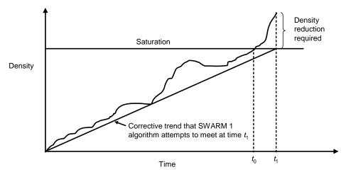
Figure 3-11. Principles of SWARM 1 ramp metering algorithm.
