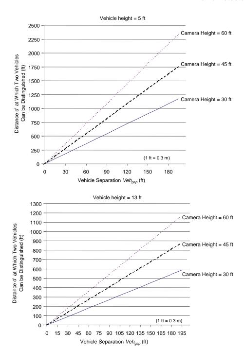
Figure 2-56. Distance *d* along the roadway at which a VIP can distinguish vehicles: (top) vehicle height = 5 ft (1.5 m), (bottom) vehicle height = 13 ft (3.9 m). These values may be further limited by road configuration, congestion level, vehicle mix, inclement weather, and pixel size.
