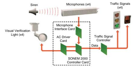
Figure 3-20. Sound detection priority system for 4-way intersection control (Courtesy of Sonic Systems, Vancouver, British Columbia, Canada).
