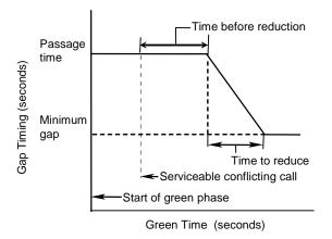
Figure 4-3. NEMA gap reduction procedure.
