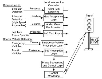
Figure 3-3. Data processing at an intersection with isolated intersection control.
