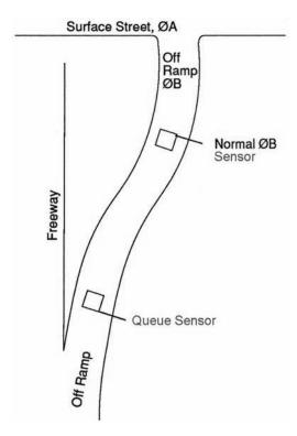
Figure 4-32. Queue discharge system.
