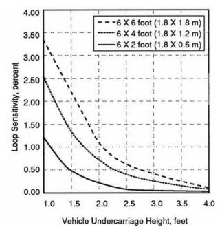
Figure 2-11. Calculated sensitivity of three-turn inductive loops as a function of vehicle undercarriage height.
