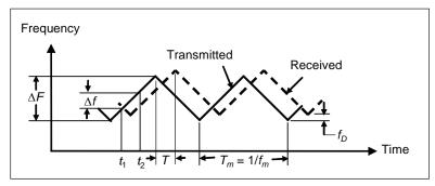
(a) Frequency modulated continuous waveform
