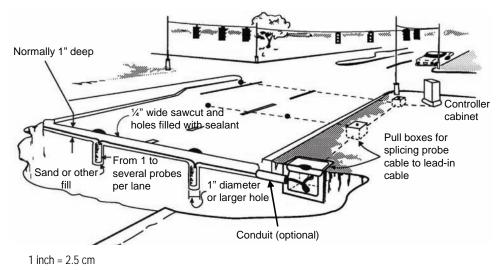
Figure 2-39. Magnetic sensor installation.
