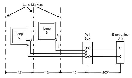
Figure 2-19. Two inductive loops connected in series to a pull box and electronics unit.
