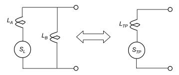
Figure 2-16. Equivalent total inductance from two inductive loops in parallel.
