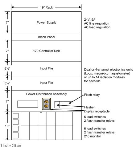
Figure 2-37. Type 170 cabinet layout (California).
