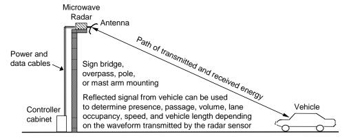
Figure 1-7. Microwave radar operation.
