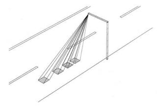
Figure 2-68. Multiple detection zone configuration in a passive infrared sensor.
