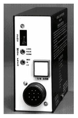
Figure 2-31. Shelf-mounted NEMA electronics unit.
