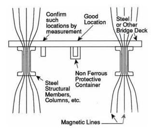
Figure 4-34. Typical installation of magnetometers on a bridge deck.
