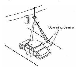
Figure 1-9. Scanning infrared laser radar two-beam pattern across a traffic lane (Drawing courtesy of Schwartz Electro-Optics, now OSI Laserscan, Orlando, FL).
