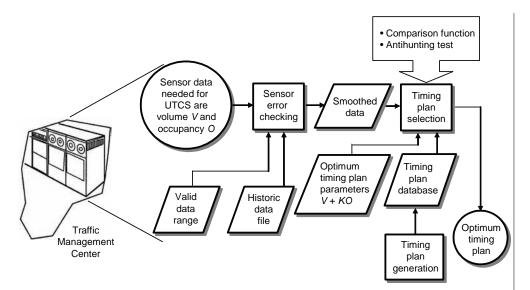
Figure 3-6. UTCS timing plan selection procedure.
