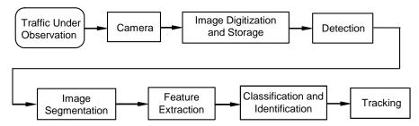
Figure 2-52. Conceptual image processing for vehicle detection, classification, and tracking. (Source: L.A. Klein, *Sensor Technologies and Data Requirements for ITS* (Artech House, Norwood, MA, 2001)).
