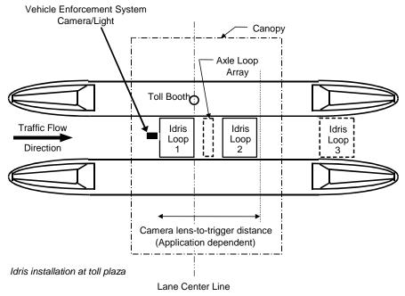
Figure 2-30. Axle location and vehicle classification using an array of inductive loops (Drawing courtesy of Peek Traffic, Inc.–Sarasota, Sarasota, FL).
