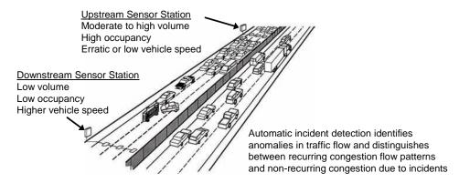
Figure 3-8. Freeway incident detection scenario.
