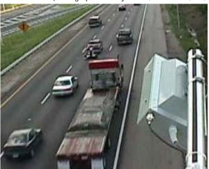
SAS-1 acoustic sensor (Photograph courtesy of SmarTek Systems, Woodbridge, VA). Figure 2-73. Acoustic array sensors.
