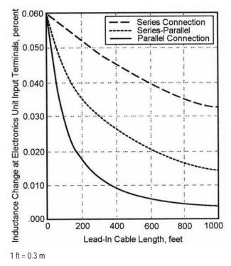
Figure 2-26. Inductance change produced by a small motorcycle as a function of lead-in cable length for series, parallel, and series-parallel connections of four 6- x 6-ft loops.
