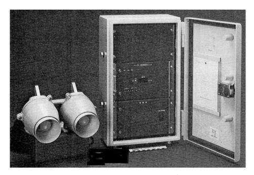
Figure 2-71. Speed-measuring RDU-101 Doppler ultrasonic sensor (manufactured by Sumitomo Electric, Japan) with separate transmitting and receiving transducers, as shown in the left portion of the figure. The cabinet on the right contains the electronic systems needed to supply power and control signals to the transducers, receive the data, and interface with the highway infrastructure.
