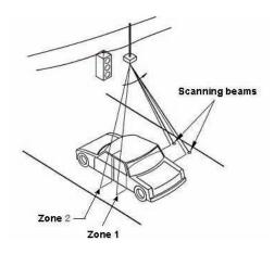
Figure 2-61. Laser radar beam geometry (drawing courtesy of Schwartz Electro-Optics, now OSI Laserscan, Orlando, FL).
