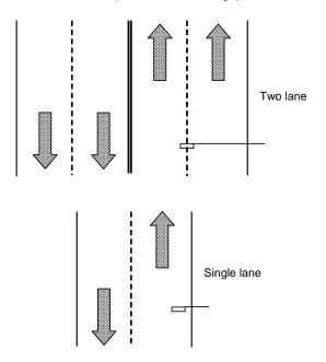
Figure 4-38. Magnetic probe placement for a single-lane and two-lane approach to a stopline.
