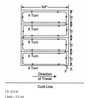
Figure 4-31. Bicycle lane loop layout with side-by-side quadrupoles.
