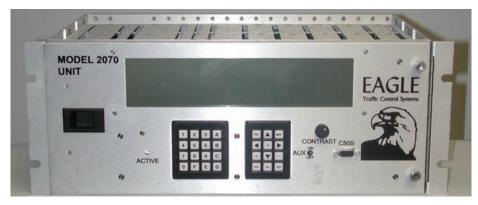
Figure 2-38. Model 2070 controller. The 2070 ATC controller is manufactured by Econolite, Eagle, Naztec, Safetran, GDI Communications, and McCain Traffic Supply at present.
