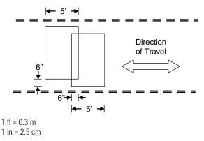
Figure 3-28. Directional detection using point sensors.
