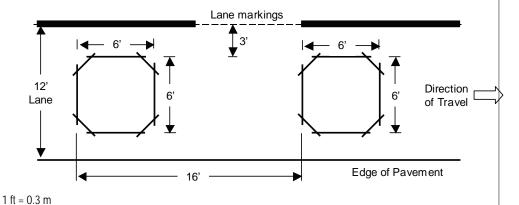
Figure 3-1. Vehicle speed measurement using two inductive-loop detectors placed a known distance apart.
