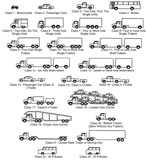
Figure 2-29. Classes available from inductive-loop classifying sensor (Source: *Model IVS-2000 Installation and Operation Manual*, Rev. 1.53 (Intersection Development Corp, Downey, CA, Sept. 1997)).
