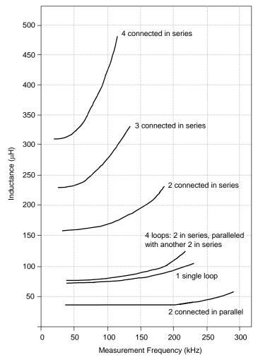
Figure 2-6. Average values of loop inductance vs. measuring frequency for series, parallel, and series-parallel connections of 6- x 6-ft (1.8- x 1.8-m) inductive loops.
