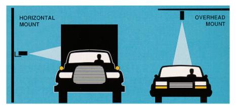
Figure 2-70. Mounting of ultrasonic range-measuring sensors (Illustration courtesy of Microwave Sensors, Ann Arbor, MI).
