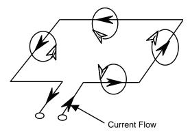
Figure 2-2. Magnetic flux around loop. The black arrows represent the current flow in the wire and the white arrows the induced flux as determined by the right hand rule.
