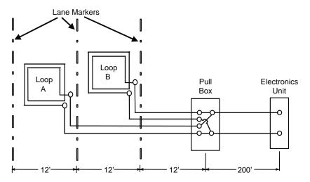
Figure 2-21. Two inductive loops connected in parallel to a pull box and electronics unit.
