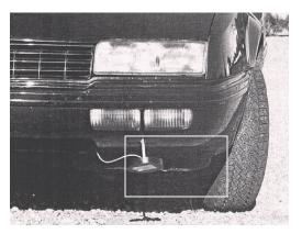
Figure 3-17. Transmitter mounted under a vehicle identifies it to a subsurface inductive-loop detector.
