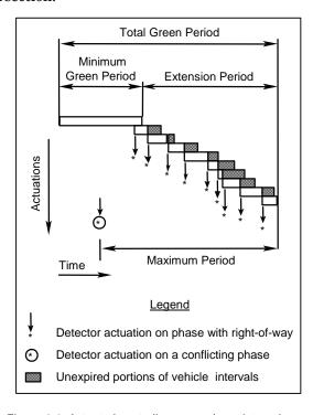
Figure 4-1. Actuated controller green phase intervals.
