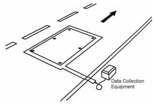
Figure 2-23. Typical installation of mat-type temporary inductive-loop detector.
