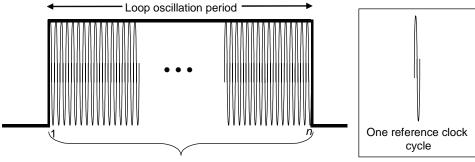
Number *n* of reference clock cycles that corresponds to the loop oscillation period
