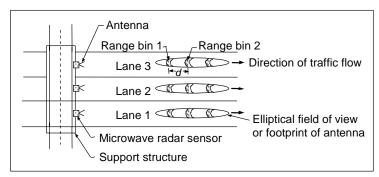
(b) Range binned footprints of radar sensors in traffic lanes
