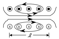
Figure 2-3. Magnetic flux for solenoid (coil). The black arrows represent the current flow, while the circles with the black and "X" centers represent the induced flux flow out of and into the plane of the figure, respectively.
