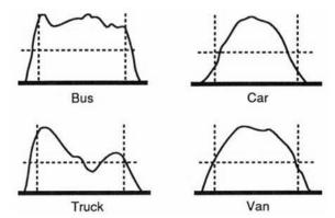
Figure 3-19. Representative vehicle signatures obtained from loops excited by high frequency signals from specialized electronics units.
