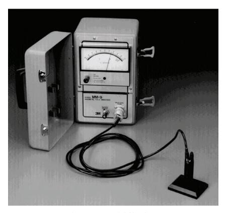
Figure 4-35. Magnetic field analyzer.
