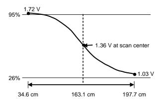
Figure 3-33. Output voltage generated by passive lane positioning sensor.
