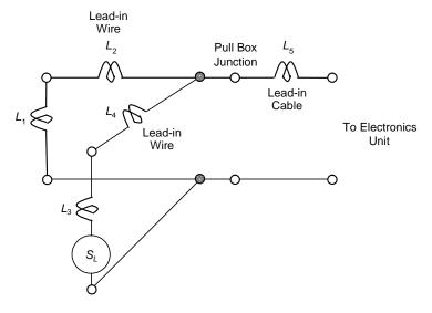
Figure 2-22. Equivalent electrical circuit for two loops connected in parallel to a pull box and electronics unit.
