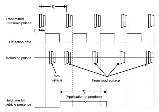
Figure 2-72. Operation of range-measuring ultrasonic sensor.
