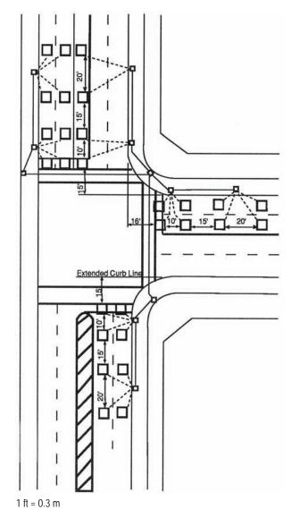
Figure 4-13. PennDOT short inductive-loop configurations.
