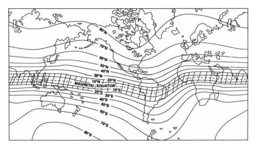
Figure 2-41. Equatorial belt showing where Earth's magnetic field is too small for deployment of simple vertical axis magnetometers between 20 degrees north and 20 degrees south of the Equator.
