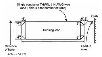
Figure 4-14. Wide inductive-loop detector layout.
