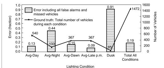
Figure 2-54. VIP vehicle count errors under varying illumination conditions. Low camera sensitivity, improper focal length of lens, low camera resolution, nonideal camera mounting height, inadequate video signal, and lack of sun shade contributed to degraded performance (source: *Traffic Surveillance and Detection Technology Development: Phase II and III Test Results, Troy, MI*, JPL Pub. D-15779 (California Institute of Technology, Jet Propulsion Laboratory, Pasadena, CA, May 1998)).
