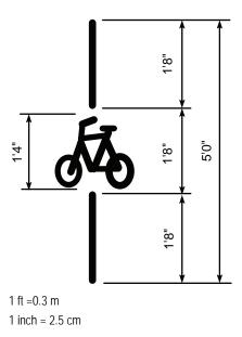
Figure 4-25. Special bicycle pavement marking used in San Luis Obispo, CA.
