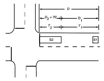
Figure 4-21. Extended call inductive-loop detector system.
