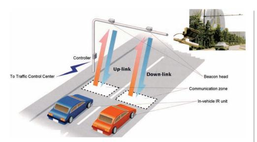
Figure 2-64. Active infrared sensor installed for transmitting traffic conditions to motorists (Photograph courtesy of Sumitomo Electric U.S.A. Inc., Santa Clara, CA).
