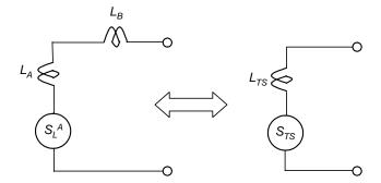
Figure 2-15. Equivalent total inductance from two inductive loops in series.
