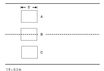
Figure 3-27. Three-loop layout for counts.
