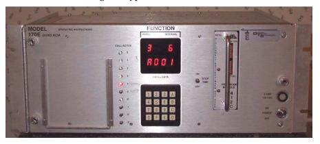
Figure 2-36. Model 170 controller (Photograph courtesy of Lawrence A. Klein).
