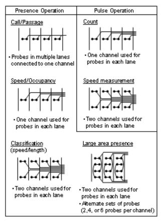
Figure 4-36. Magnetometer-probe placement in support of several data-gathering functions.
