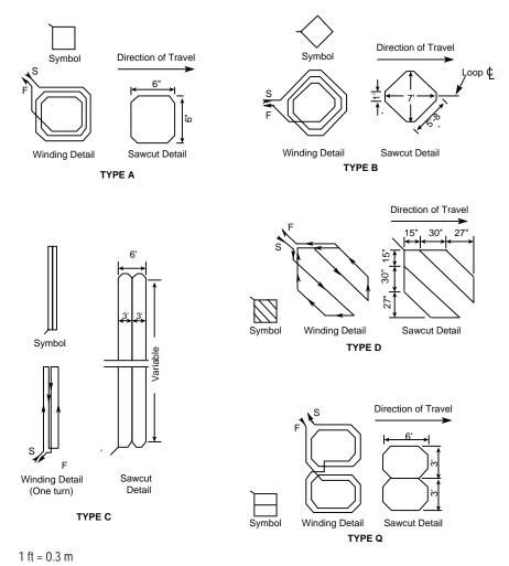
Figure 4-10. Caltrans-specified loop shapes.
