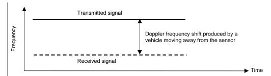
Figure 2-57. Constant frequency waveform.
