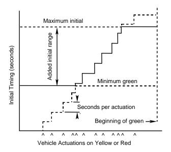
Figure 4-2. Variable initial NEMA timing for green signal phase.
