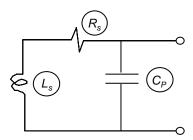
Figure 2-5. Equivalent electrical circuit for an inductive loop with capacitive coupling to the sidewalls of a sawcut slot.
