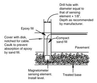
Figure 4-33. Conceptual magnetometer sensor installation.
