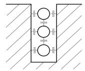
Figure 2-4. Capacitive coupling between the loop wires themselves and the sawcut slot sidewalls.
