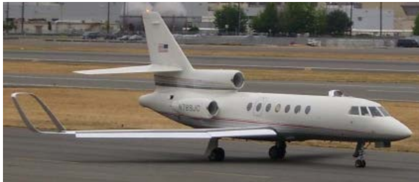
Figure 3. Test Aircraft with Spiroid Winglets Installed
