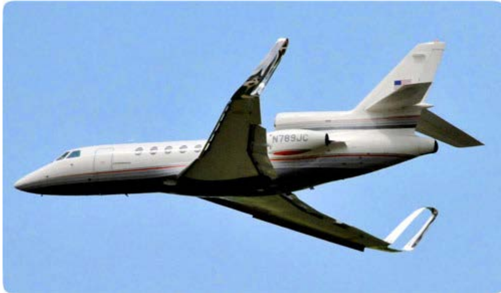
Figure 1. Aviation Partners' Spiroid Winglets Installed on a Falcon 50 Aircraft
