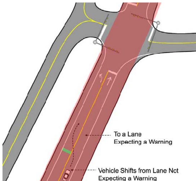
Figure 4. Geometry of Tests for Late Lane Shift Warning
