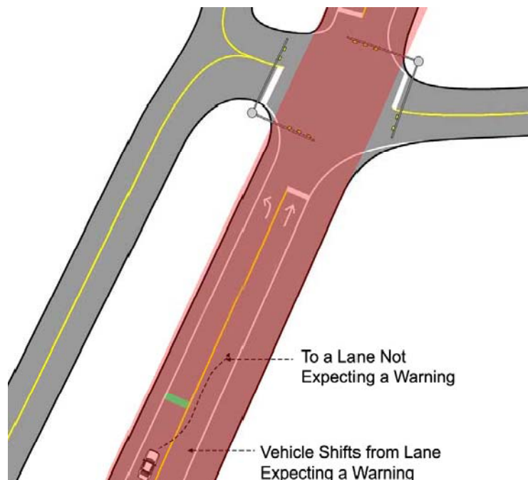
Figure 5. Geometry of Tests for Late Lane Shift Nuisance Warning
