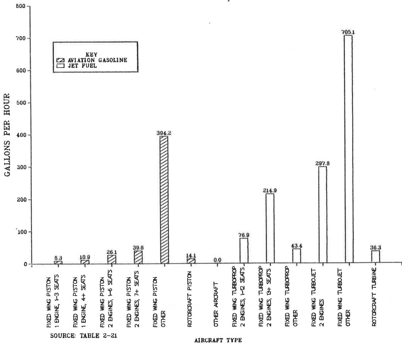
FIGURE 1-6. 1982 MEAN FUEL CONSUMPTION RATES BY AIRCRAFT TYPE
