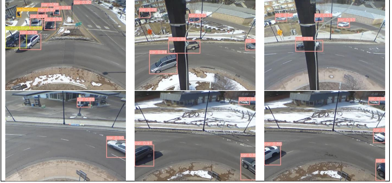
Fig. 5.4: Detection occlusion cases for YOLO8s multi-image detection. TOP: vehicle queuing, foreground occlusions, BOTTOM: vehicle edge detection
