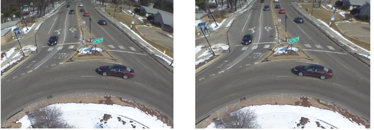
Fig. 4.3: Input image (left) and the rectified image calibration result.(right)
