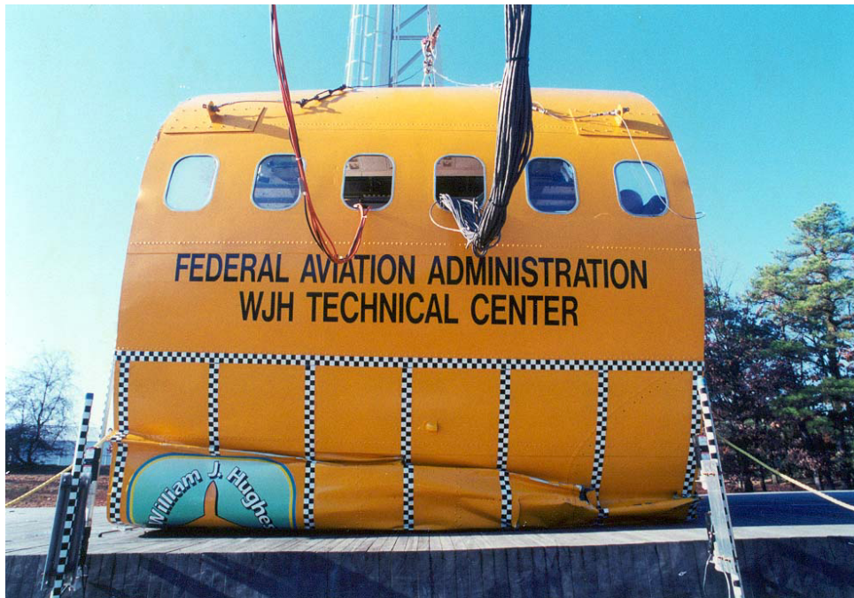
FIGURE 51. LEFT VIEW—BUCKLE OF THE FUSELAGE SKIN
