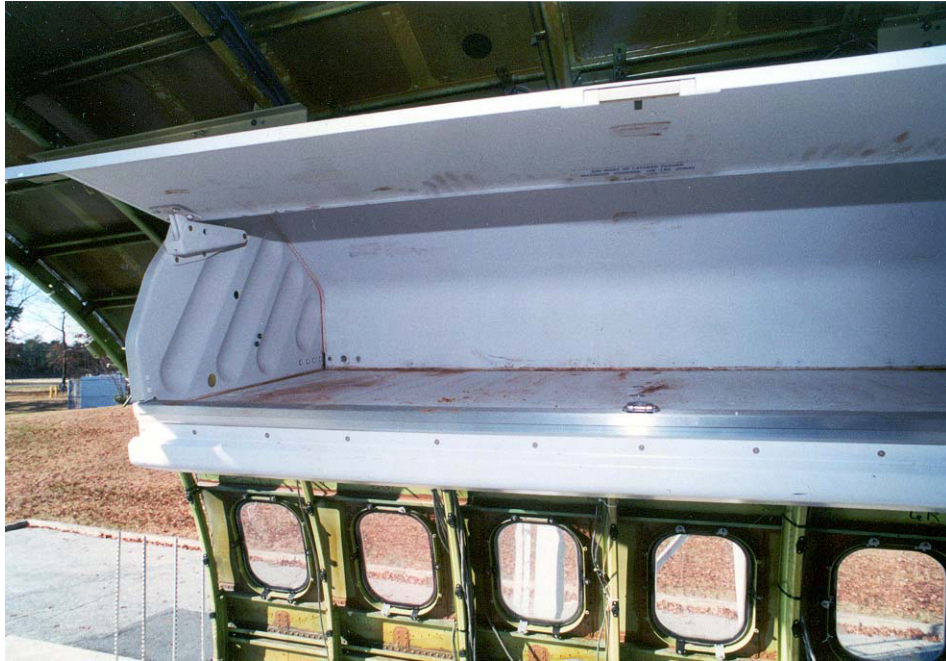
FIGURE C-52. HEATH TECNA BIN—OPEN FRONT
