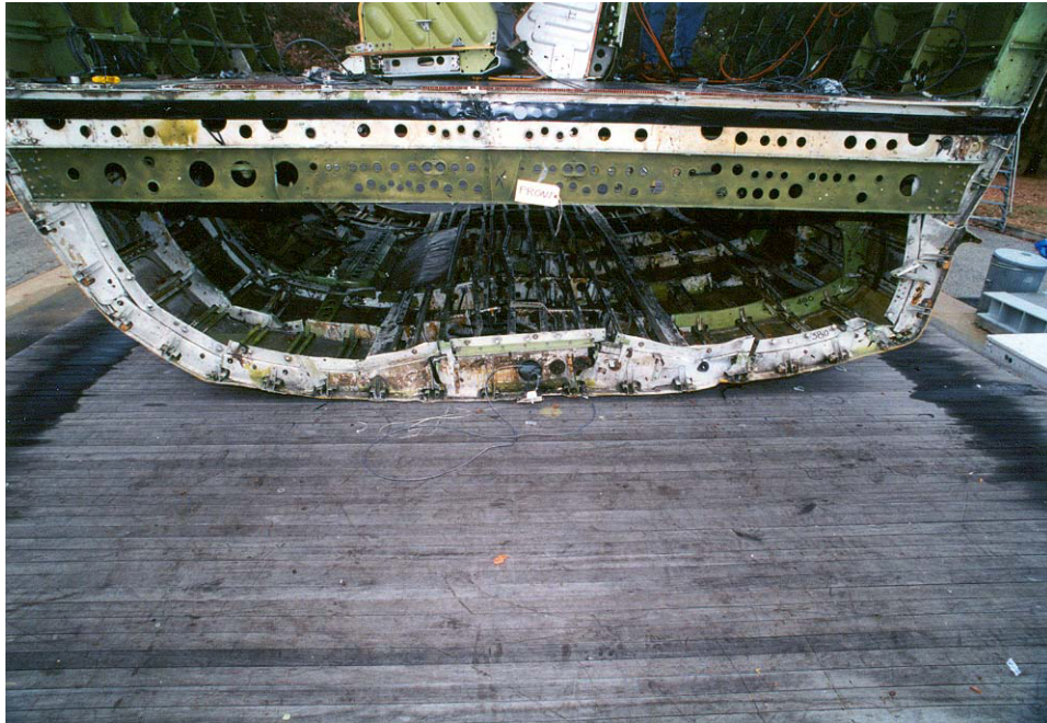
FIGURE C-71. CARGO CABIN FLOOR BUCKLE—FRONT
