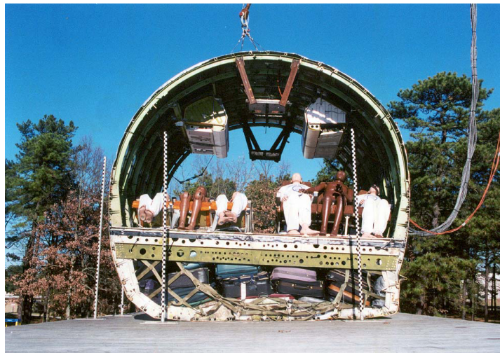
FIGURE 50. CARGO AREA DEFORMATION
