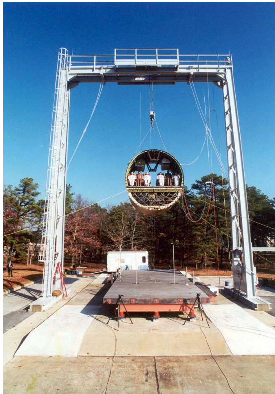
FIGURE C-2. DYNAMIC DROP TEST FACILITY
