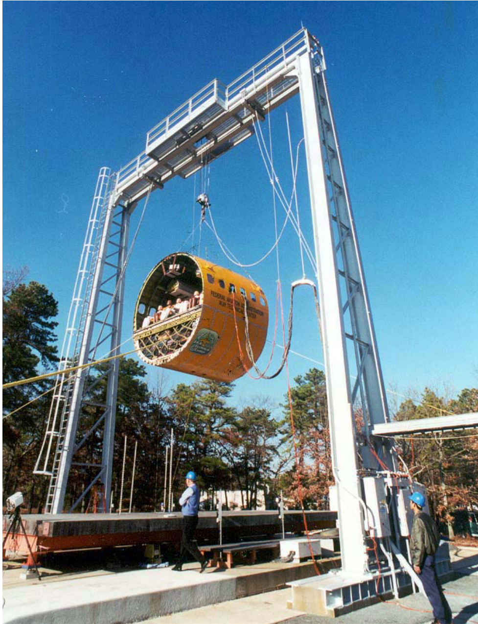
FIGURE 2. DYNAMIC DROP TEST FACILITY AND TEST FUSELAGE SECTION
