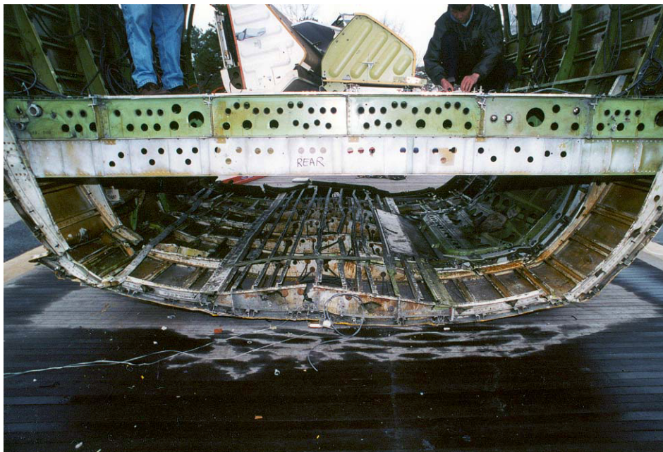
FIGURE C-72. CARGO CABIN FLOOR BUCKLE—REAR
