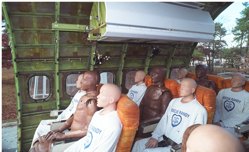
FIGURE 19. ATD LOCATION—RIGHT SIDE
