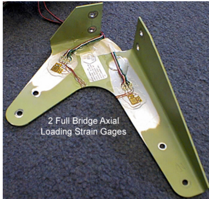
FIGURE 16. STRAIN GAGE BRIDGE LOCATION—HT5 THROUGH HT9
