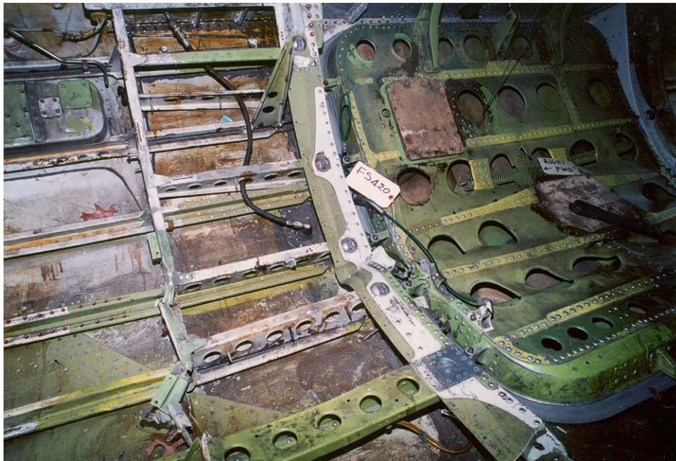
FIGURE C-78. CARGO DOOR—RIGHT FRONT
