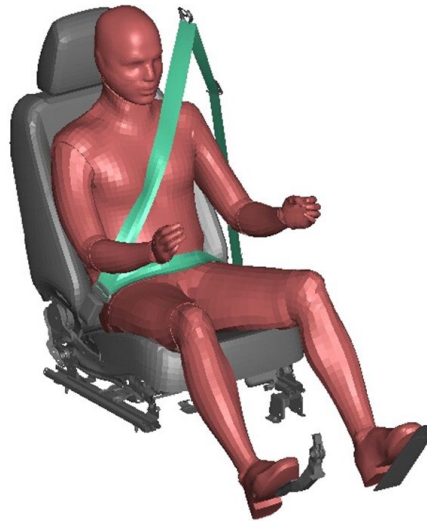
Figure 6. Demonstration of a proper routing of the seat belt on the M50-OS model
