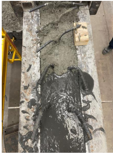
Figure 16. UHPC-SCC interface after casting
