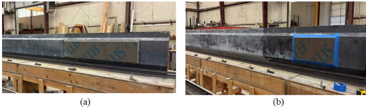
Figure 10. Formwork side after placement of (a) 5 ft wooden web insert and (b) 3 ft wooden web insert
