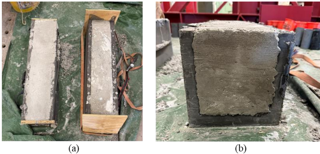
Figure 21. (a) Completed UHPC shell specimens and (b) end view of UHPC shell specimen
