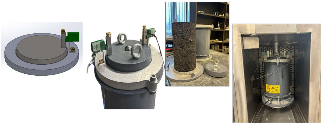
Figure 19: Triaxial resilient modulus testing setup.
