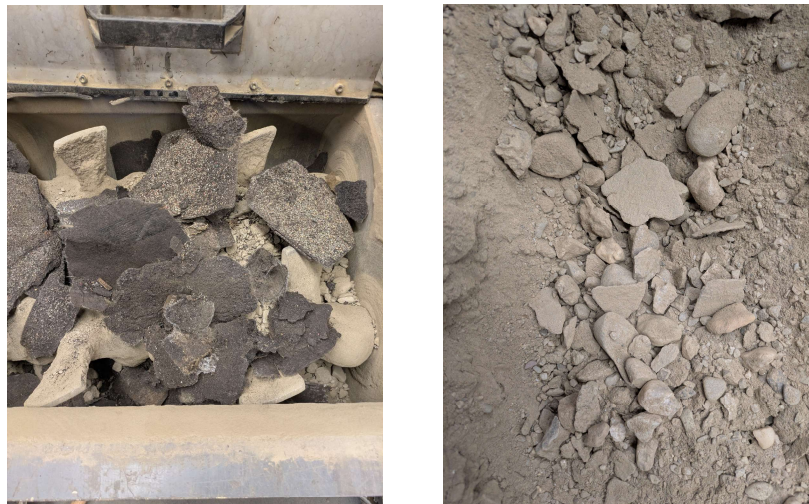
Figure 34: FDR + minimally processed RAS before mixing (left) and after mixing (right).
