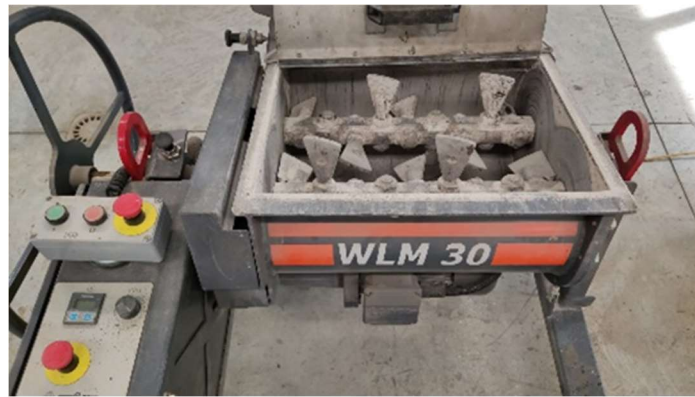
Figure 16: Wirtgen pugmill WLM 30 mixer.
