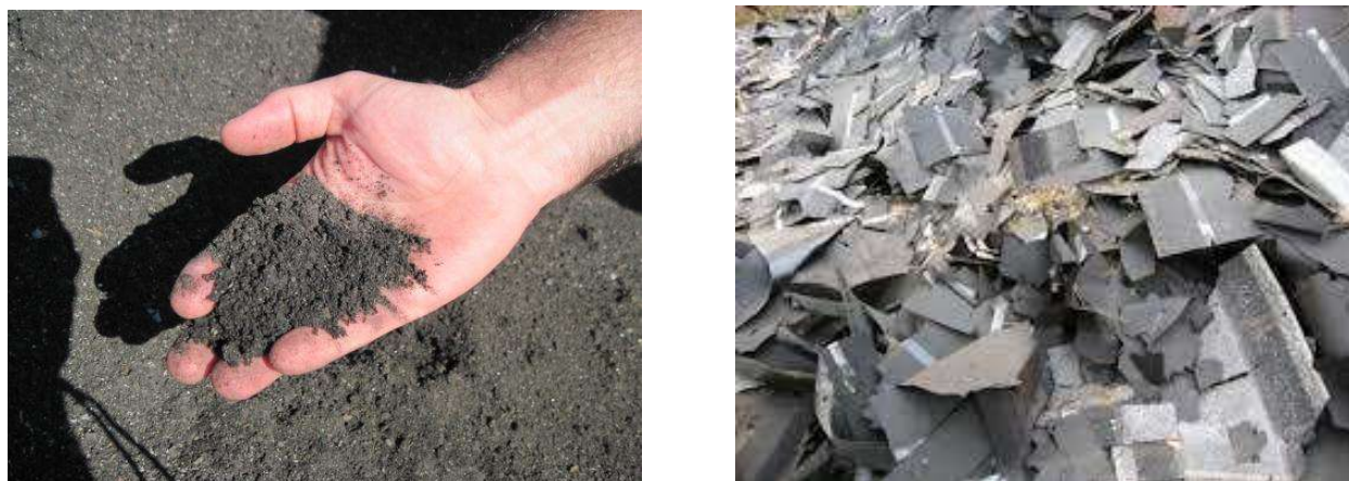
Figure 6: Processed (left) and unprocessed (right) RAS.
