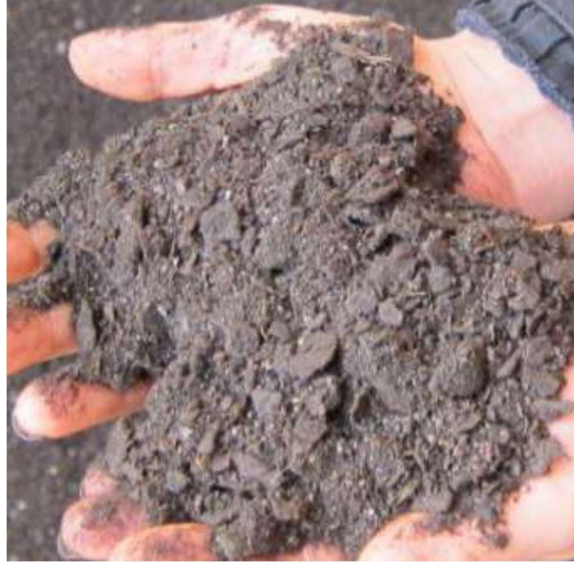
Figure 1: Potential challenge of “corn flake” shingles. (Willis, 2013)
