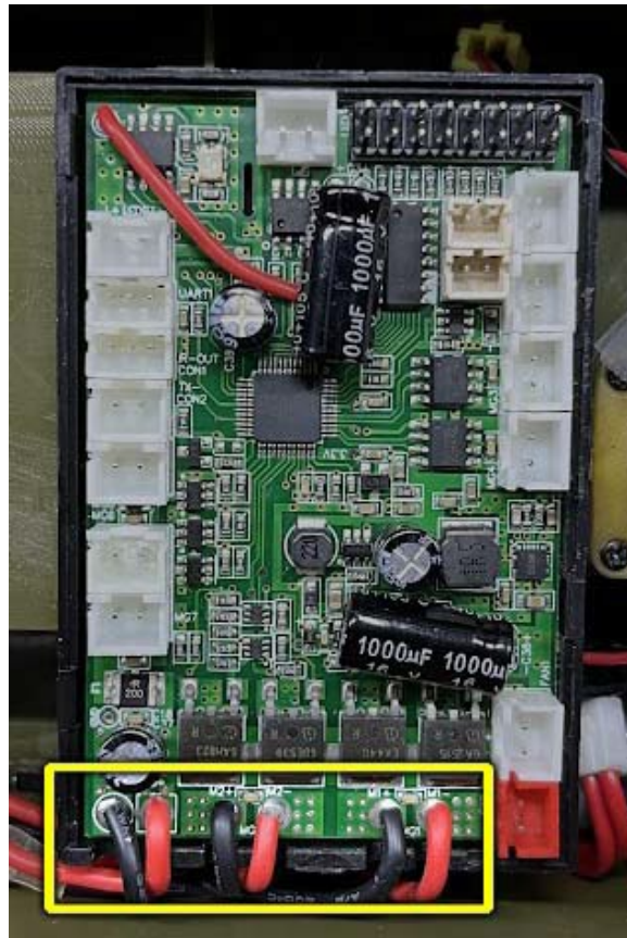
Figure 99 Soldered power connections to cut on stock control board (Gamble 2025a)
