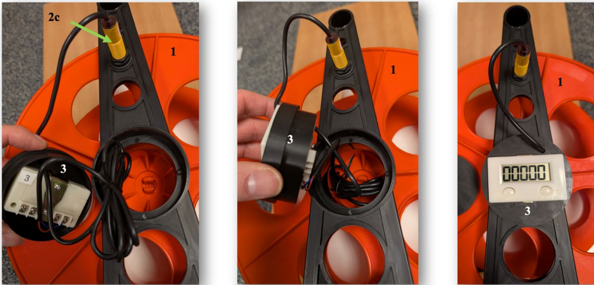
Figure 82 Coil wire and insert counter into reel
