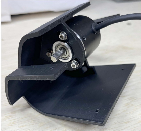
Figure 106 Left encoder secured in housing (Gamble 2025a)
