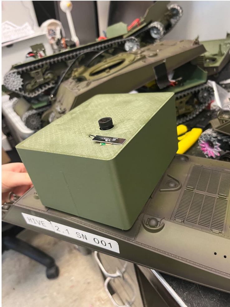
Figure 44 Antenna placement on turret box
