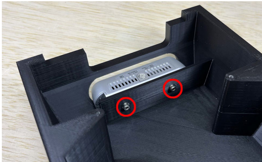
Figure 110 Underside of shell with RealSense mounted. Mounting screws highlighted (Gamble 2025a)
