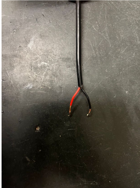
Figure 64 Two wire black connection cable with stripped end
