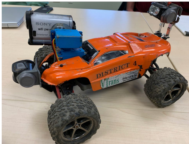
Figure 2 HIVE 1.0 used by VTrans with articulated Sony Action Cam video camera mounted on two servo motors (Burton 2020)
