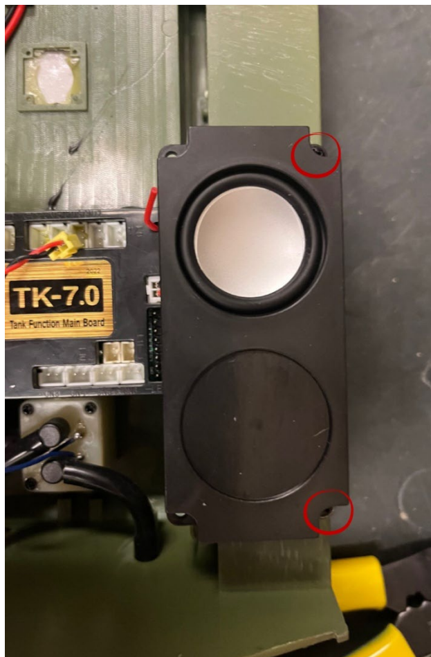
Figure 50 Remove two screws and speaker
