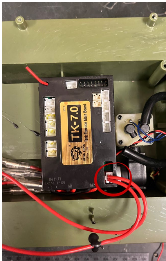
Figure 51 TK-7.0 board with one set of wires remaining
