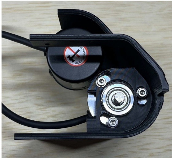
Figure 107 Right encoder secured in housing. (Gamble 2025a)
