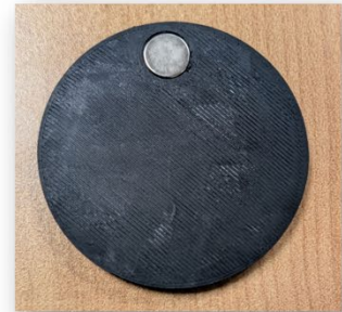
Figure 76 Insertion of magnet into magnet holder for reel rotation counter
