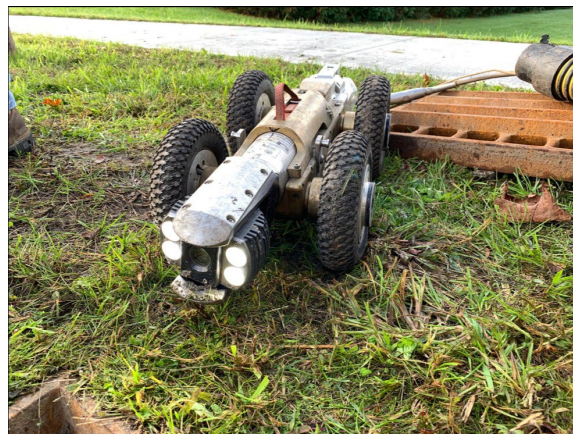
Figure 9 Commercial inspection vehicle used by VTrans (Burton 2020).
