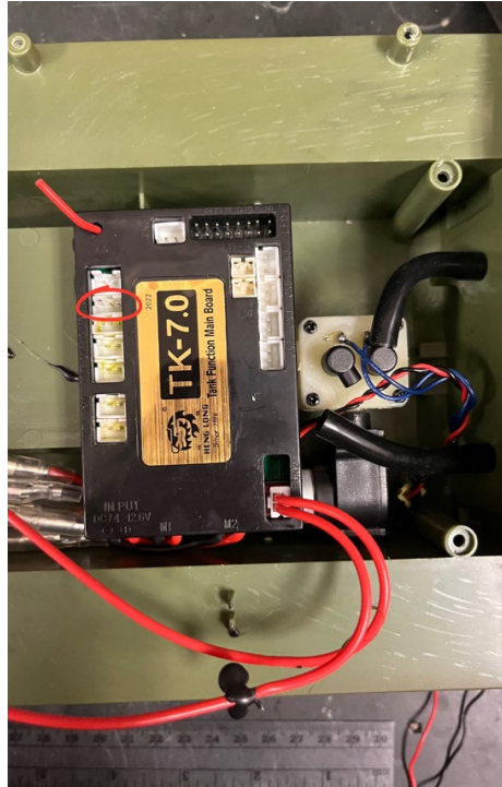
Figure 62 TK-7.0 board with 3.3V port circled
