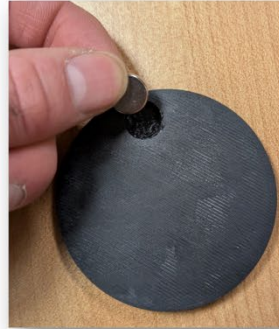
Figure 76 Insertion of magnet into magnet holder for reel rotation counter
