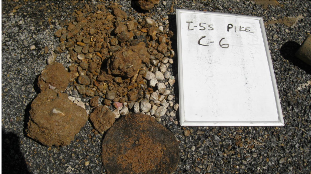
Figure 8. Example from crushed concrete layer from Core #6 (no steel bars present)
