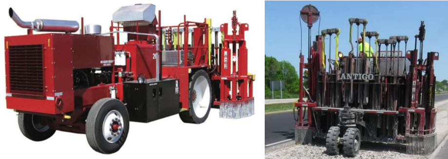
Figure 5. Variations of MHB equipment created by Antigo Construction, Inc. (21) .
