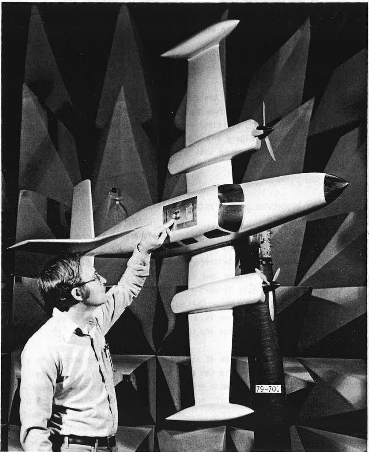
Figure 2-2 Antenna Positions on the Cessna 402B Model
