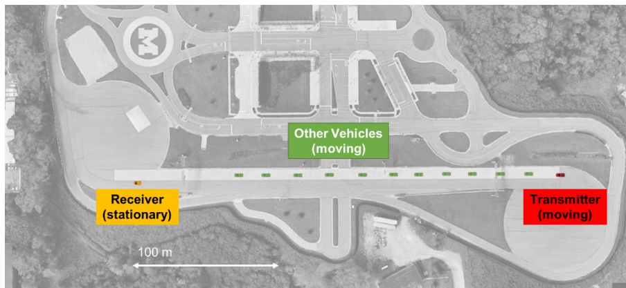
Figure 35. Light traffic scenario shows the transmitting car last in line with eleven other cars separated by approximately 20 m.
