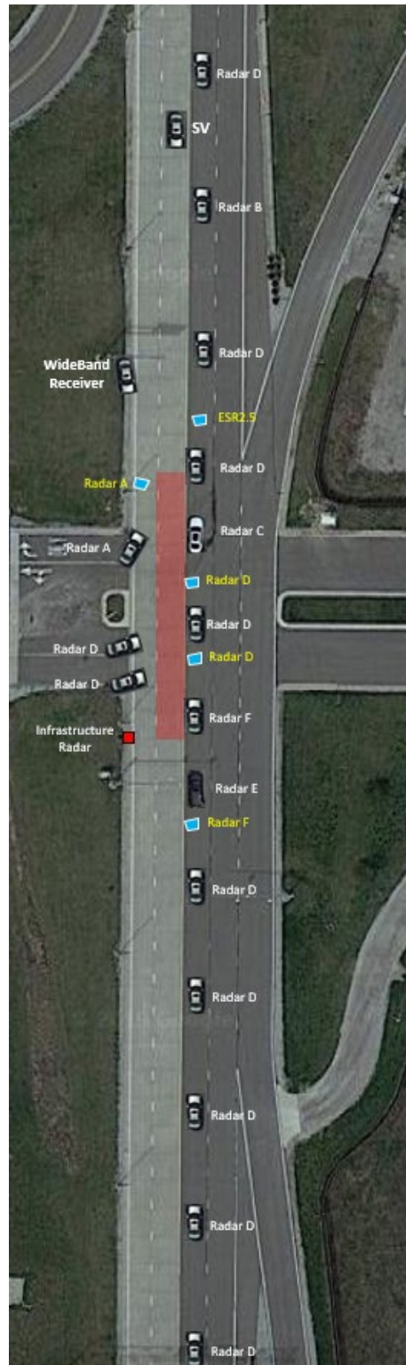
Figure 15. Location of test vehicles, interfering radars, and zone where SV encountered POV
