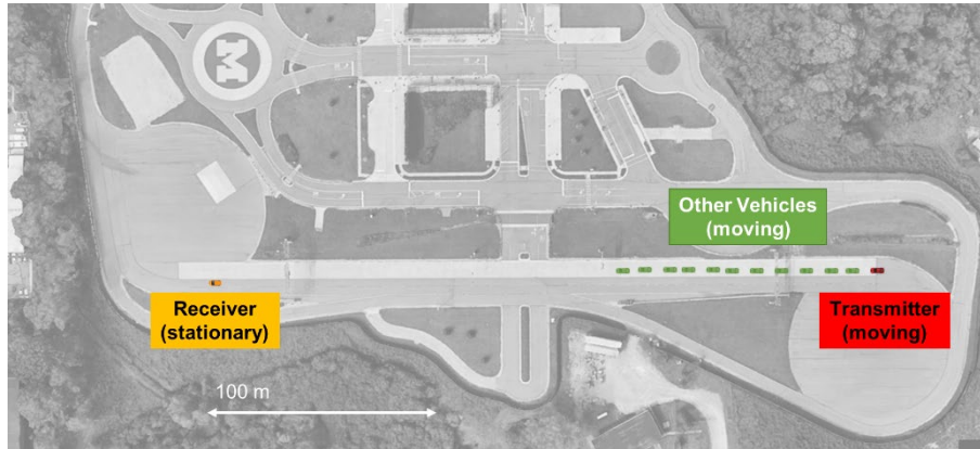
Figure 36. Heavy traffic scenario shows the transmitting car last in line with eleven other cars separated by approximately 10 m.
