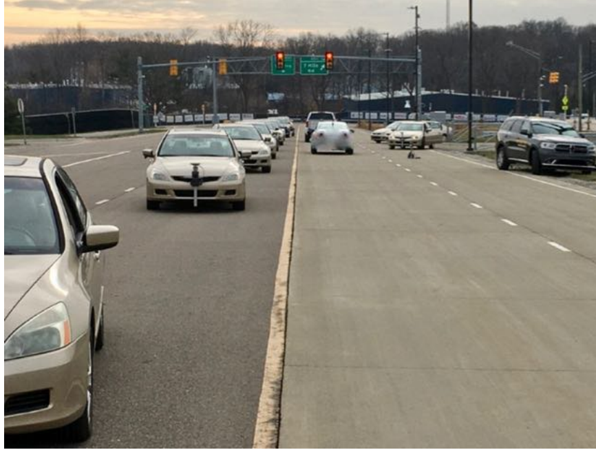
Figure 13. Test layout showing SV, POV, interfering vehicles and radars, and wideband receiver
