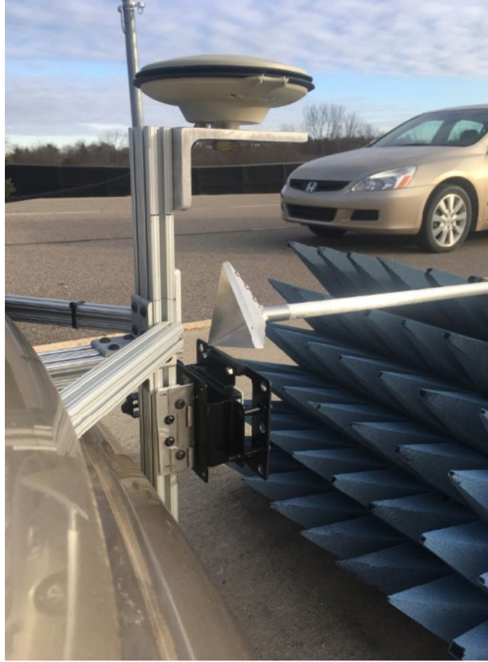
Figure 21. Survey of 10dB corner reflector location
