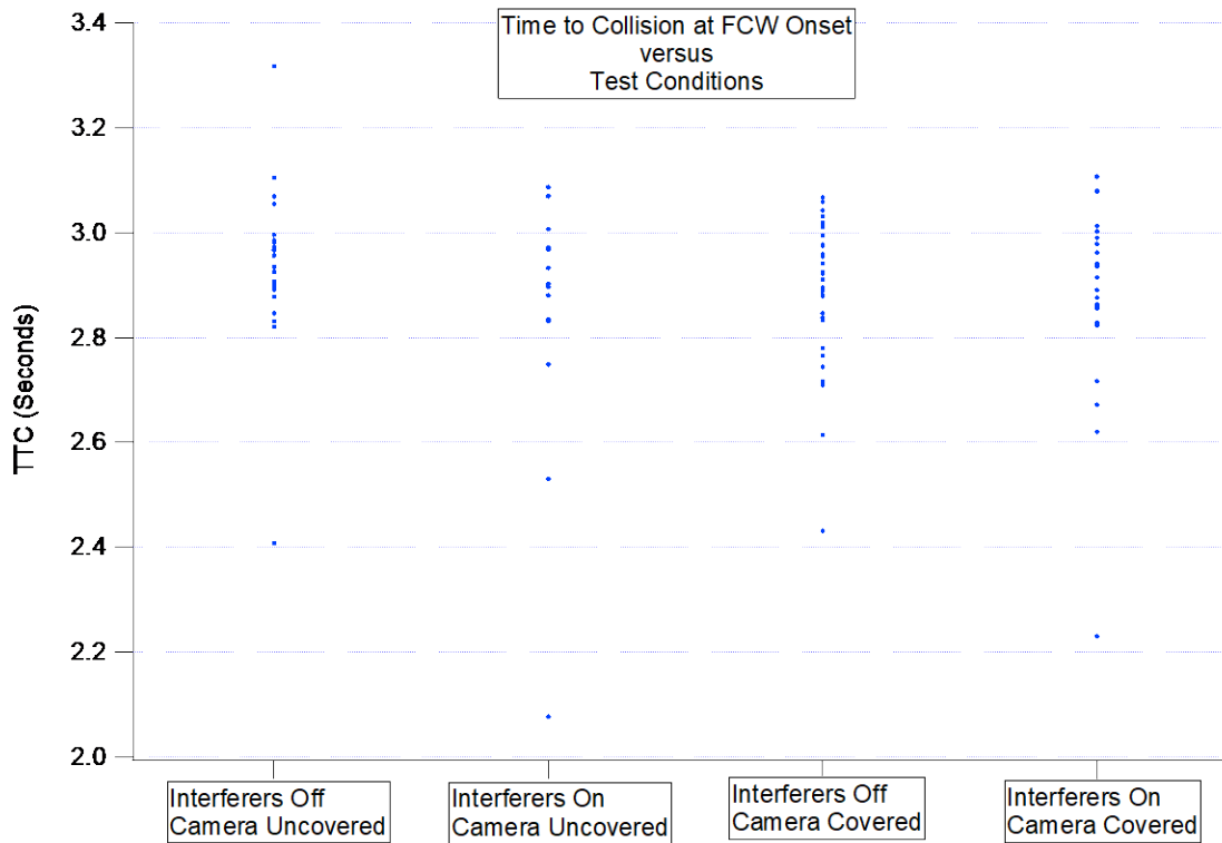
Figure 25. Time to collision at onset of forward collision warning
