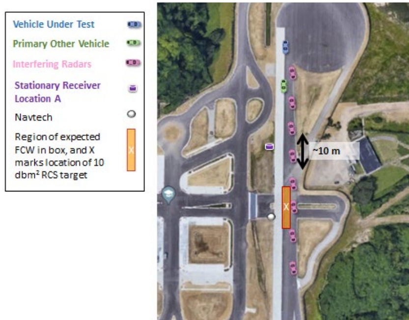
Figure 11. Aerial view of Mcity with transmitter and receiver collection geometry, as well as vehicles representative of a rural highway scenario for evaluation of system impact
