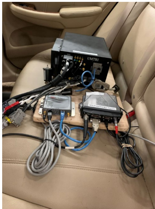
Figure 19. Data acquisition system with RTK receiver and cell modem
