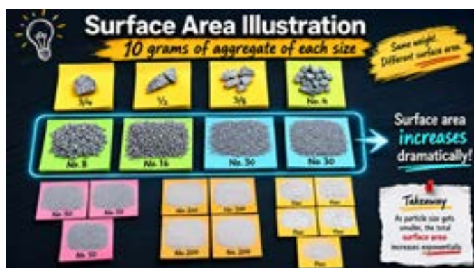
Figure 2 - Surface-area illustration of aggregate size fractions. Testing identified the intermediate fraction passing the No. 4 sieve and retained on the No. 30 sieve (4.75-0.60 mm) as the most influential portion of the gradation.
