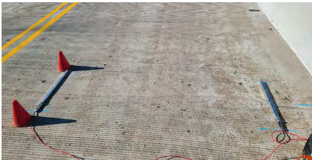
Figure 3-14. ST placement on bridge deck for live load testing.
