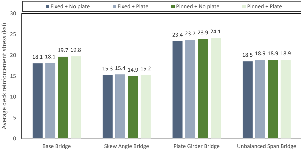
Figure 5-22. Summary of maximum average deck reinforcement stresses for all parametric models.
