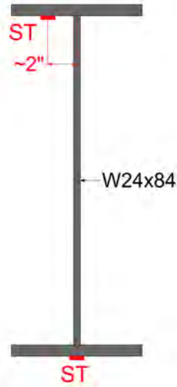
Figure 3-7. Strain transducer placement on girders.
