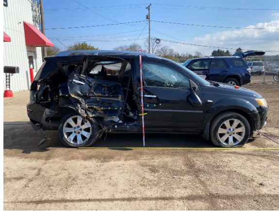
Figure 6. View of the right-side damage of the 2007 Mitsubishi Outlander
