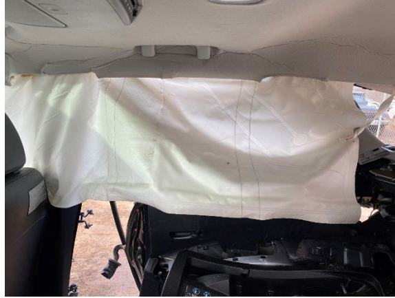
Figure 10. View of the right IC air bag deployed in the Mitsubishi
