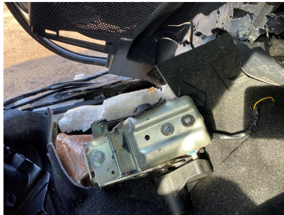
Figure 8. View of the interior of the Mitsubishi depicting the second-row right seating position track mount
