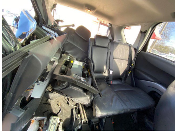
Figure 7. View of the interior of the Mitsubishi depicting the intrusion of the right rear door and shifting of the right seating position
