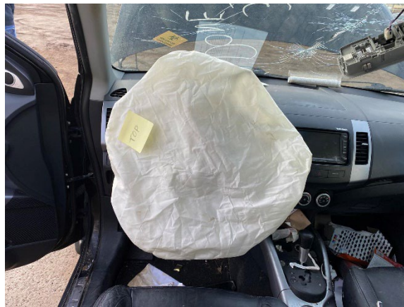
Figure 9. View of the driver's deployed frontal air bag in the Mitsubishi
