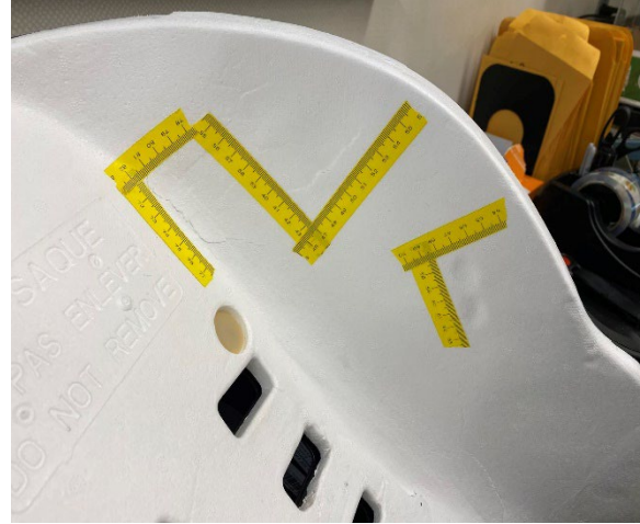
Figure 17. View of contact points on the left side of the CRS
