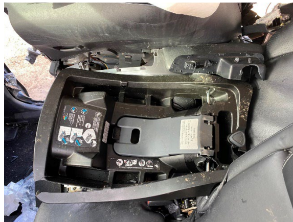
Figure 18. CRS base that was secured in the second-row right seat of the Mitsubishi
