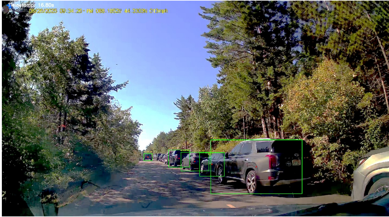
Figure 6: Computer Vision Recognition of Vehicles Parked in the Right Lane on Park Loop Road Source: Volpe Center
