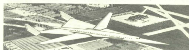
ARTIST's concept of a supersonic transport. Extensive FAA-NASA-Defense Department research is being devoted to SST problems. In this concept aircraft has variable sweep wings, swept back for cruise; forward for subsonic flight.
