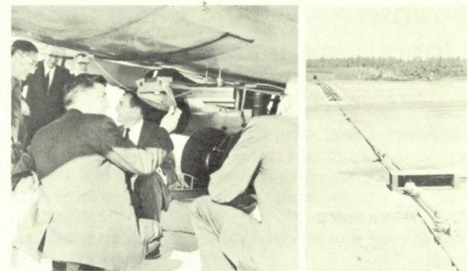
BOEING 720 jetliner racing down runway at 130 knots during test is halted in less than one fourth the normal stopping distance by pilot lowering tail hook as he nears a steel cable placed across the runway. Hook engages cable attached to loose fitting pistons in water filled tubes buried alongside runway and halts the plane early.
