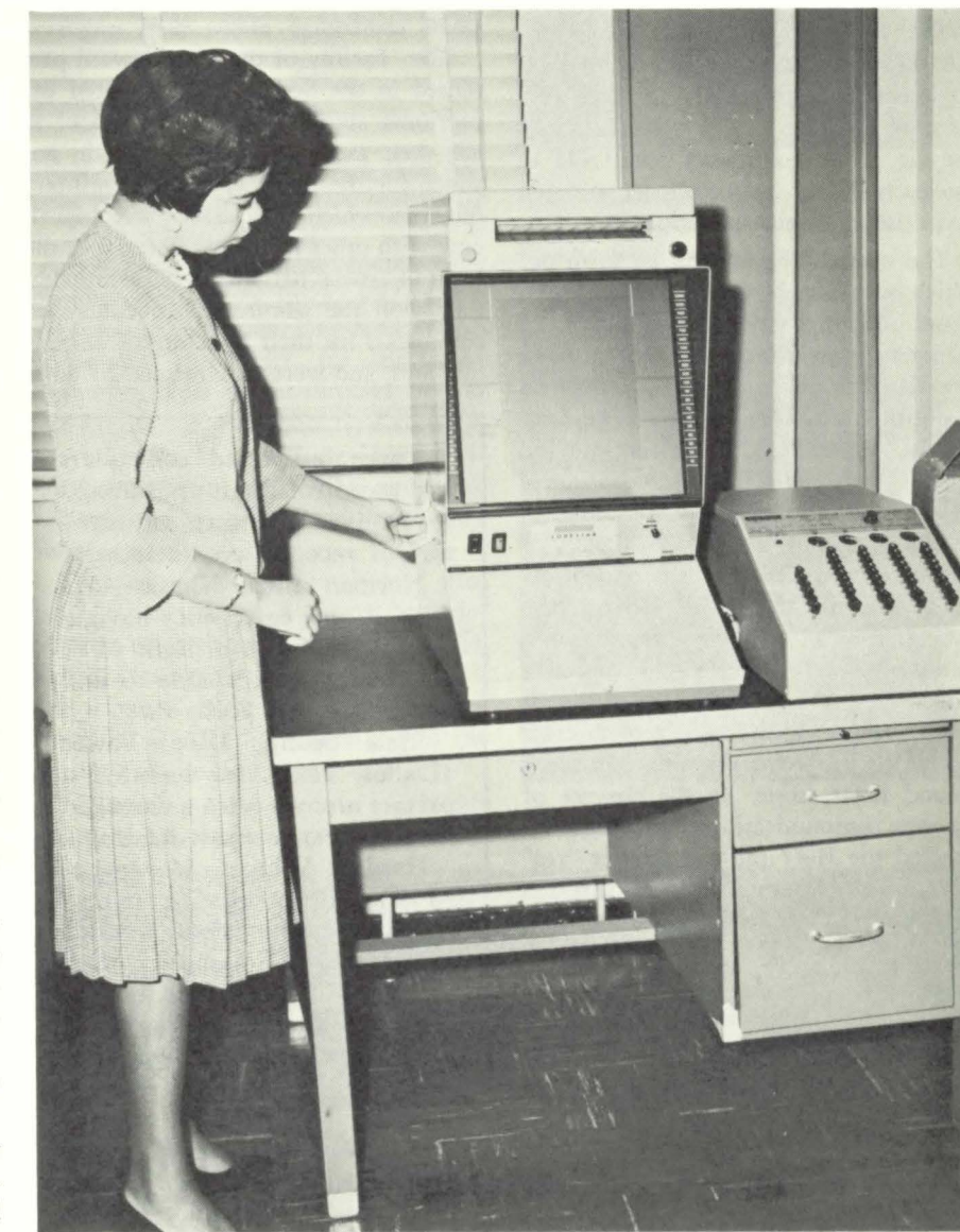
OPERATOR checks cartridge containing hundreds of microfilm shots which are located by pushing button combination on right and correct image appears on screen; push another button and a copy comes out the top in 25 seconds.
