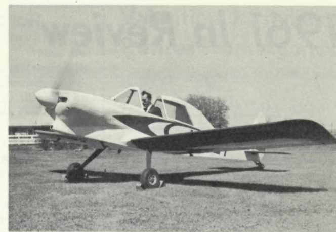
TURNER T-40 is warmed up by owner and builder E. L. Turner, an FAA aeronautical engineer with Southwest Region. Sleek craft took 2½ years and roughly $1,000 to build. It has folding wings. Builder was awarded EAA's Outstanding Design Trophy at Rockford, Ill., last August.
