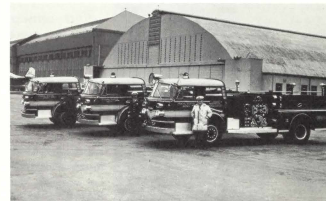
RECENT firefighting equipment received by Agency are these three 1500-gallon pumper fire trucks. One is on duty at Washington National. The other two at the new international airport at Chantilly, Virginia.
