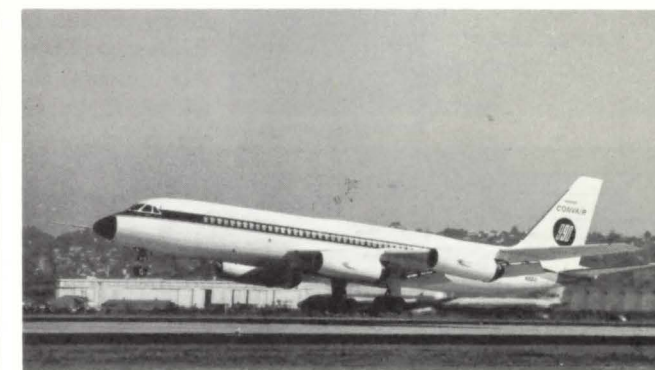
LATEST addition to U. S. passenger service is the trim Convair 990, which joined American Airlines' fleet in March. The new jet incorporates engineering advances proved out on the B-58 supersonic bomber. (Convair photo)
