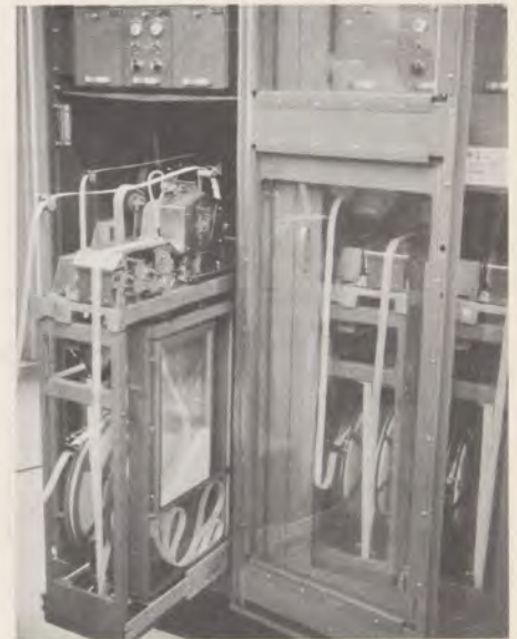
HIGH to low speed converter circuits; (right) 800 WPM high speed reperforators and 100 WPM transmitter-distributor.
