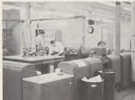
THE ADIS in Kansas City's Telecommunications Center; (center) Service "B" teletypewriter loop; (right) "A" and "C" teletypewriter loop in background with automatic relay units at right center and portion of "B" loop in foreground.
