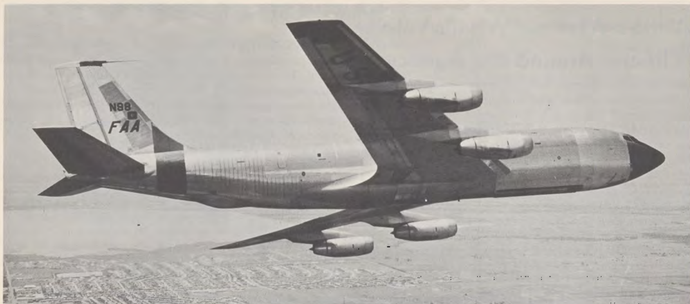
BOEING C-135 jet converted into a flying laboratory for high altitude checking of air navigational aids.
