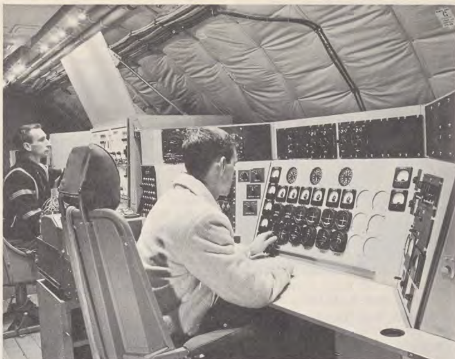
INTERIOR of C-135—Nan-98—high altitude jet which is used in nav aids inspection. Consoles indicate signal response and accuracy from ground installations.
