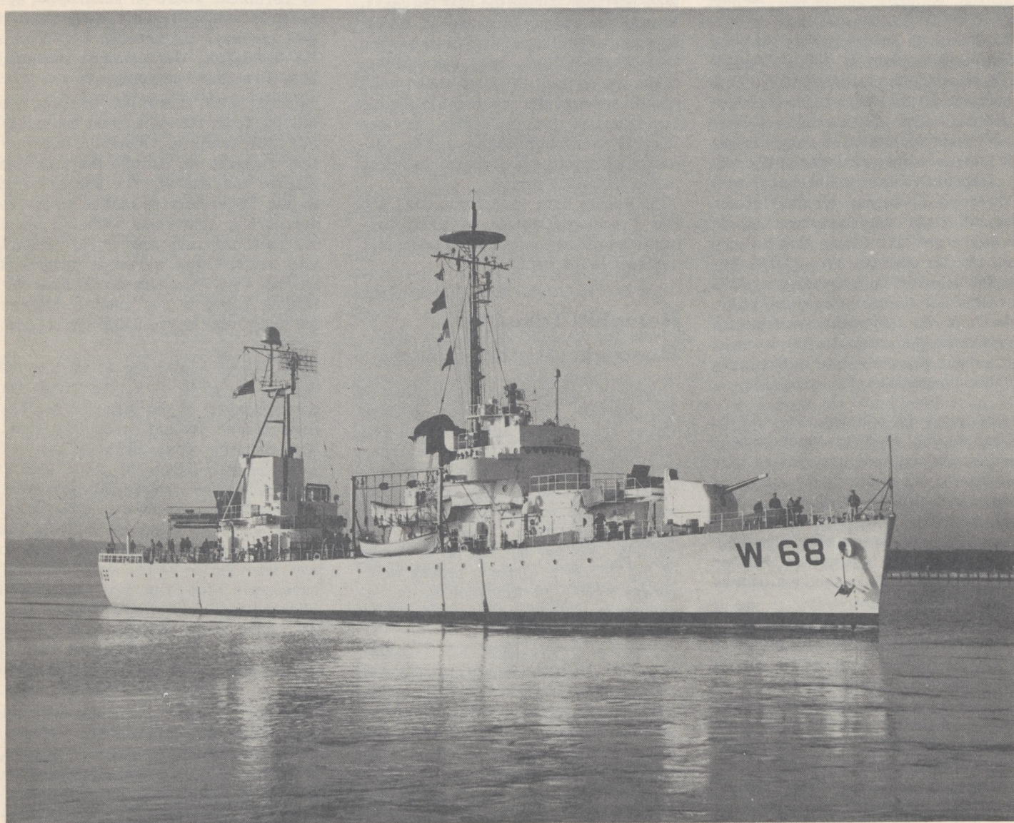
USCG CUTTER ANDROSCOGGIN with VORTAC facility aboard during test as part of an effort by the FAA and the Coast Guard to develop acceptable guidance signals for aircraft from a pitching, rolling ocean ship. VORTAC provides two sources of azimuth or bearing information.
