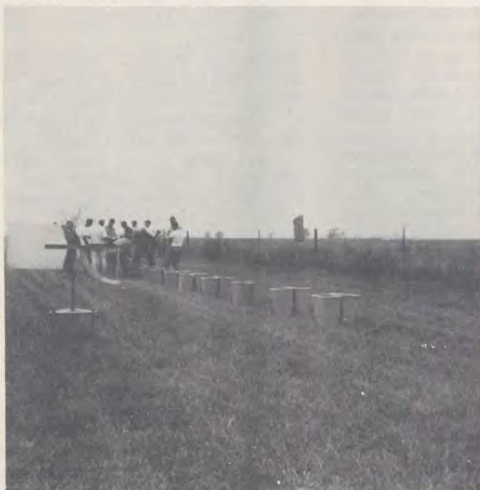
Plastic waste baskets, standing side-by-side, were used to measure swarth width. At right students load fertilizer into a Stearman.
