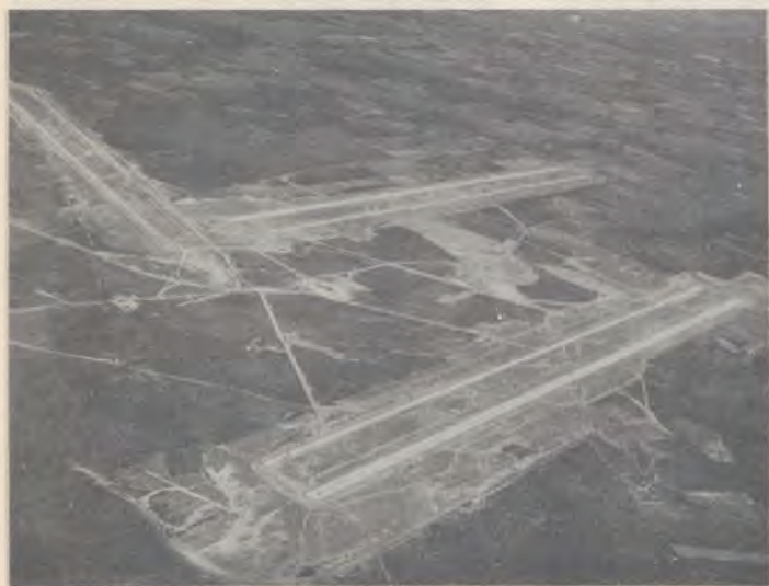
Aerial view of two parallel North-South runways which are 11,500 feet long and 150 feet wide and the 10,000 foot long and 150 foot wide Northwest-Southeast runway. Paving work called for laying about 1,196,000 square yards of Portland cement concrete.
