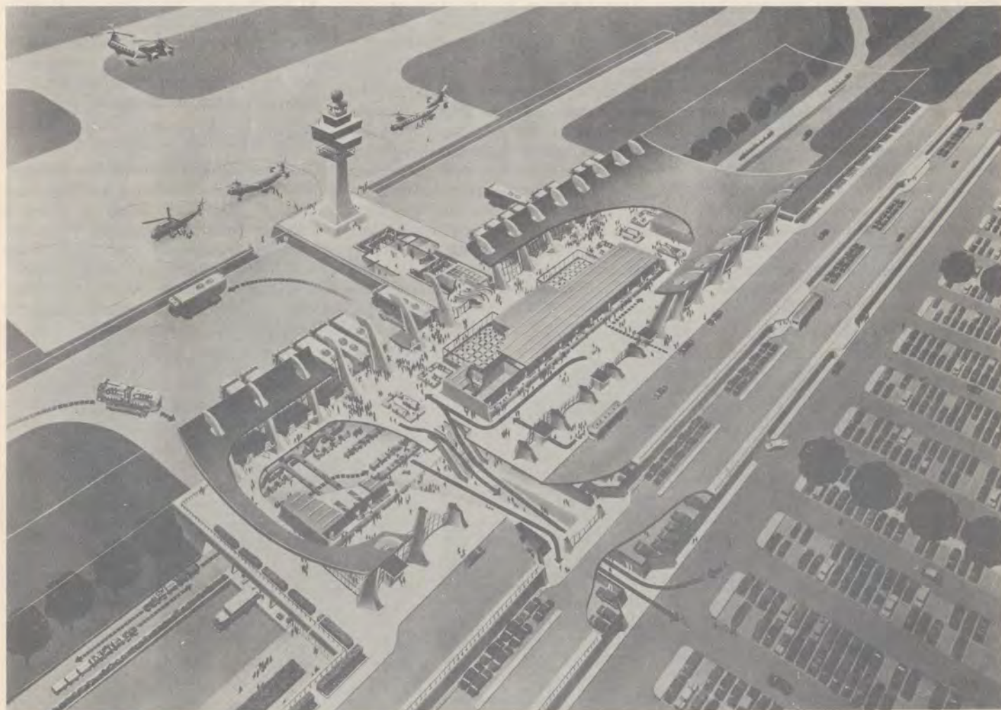
Elevation view of the futuristic, two-level building with most of its concave roof cut away to show the interior. Arrows at center indicate the routes for arriving and departing passengers, a plan designed to eliminate the confusion found in single-level terminals. Control tower will be topped by a globe which will house radar equipment.
