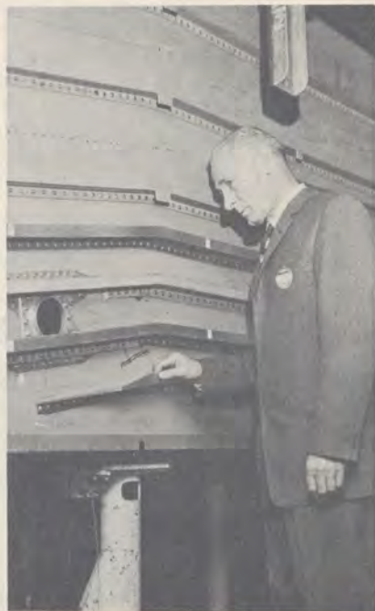
R. L. Van Note inspects for reported difficulty with cracked stringer during production of 707.
