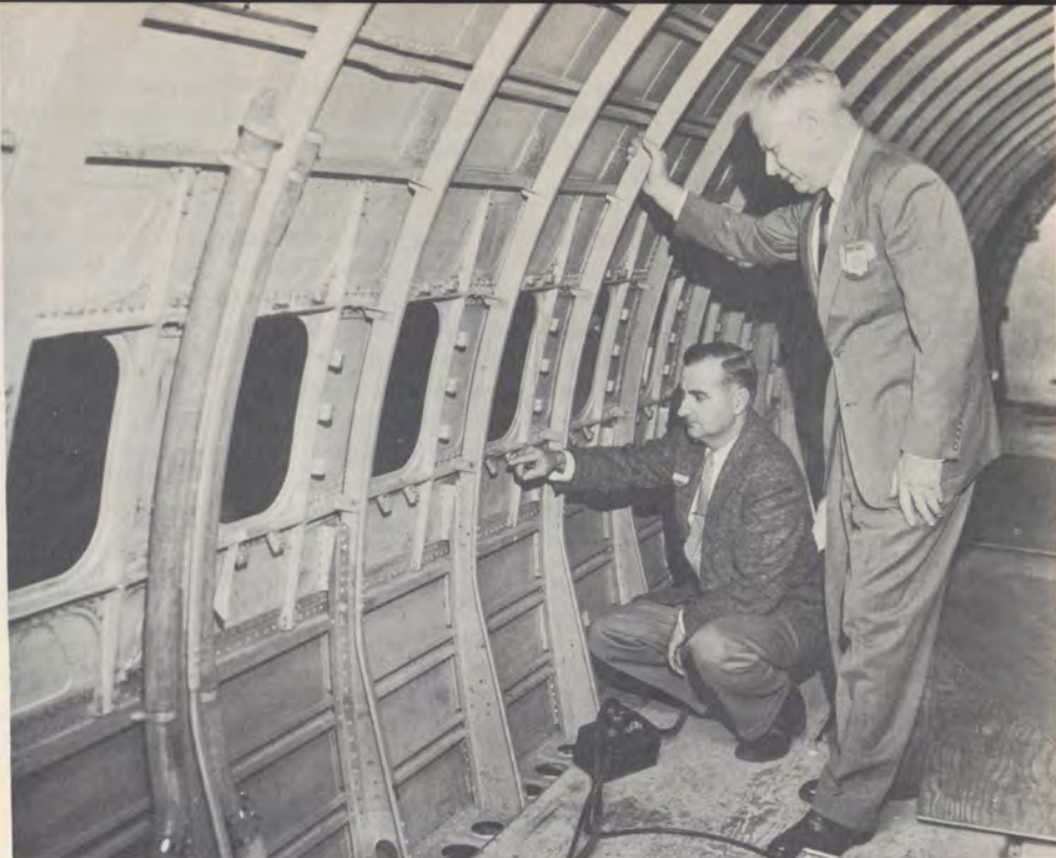
Manufacturing Inspector Leroy Gammon points out structural defect on Boeing 707 body structure to Supervising Inspector V. L. Gardner. Defect will be corrected before plane is approved.
