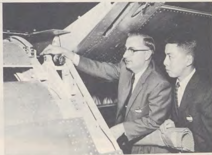
Manufacturing inspectors Leroy Gammon and Wing Chin inspect a flap carriage stop on a 707 during a regular tour of inspection.
