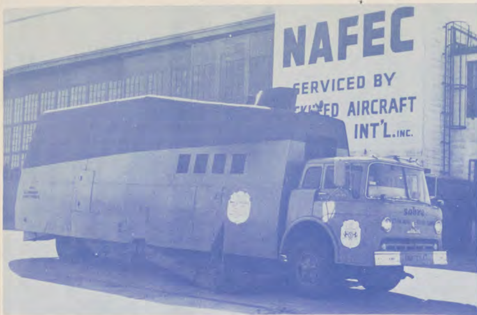
Runway vacuum cleaner picks up foreign objects before they get chance to enter jet engines.
