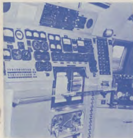
This control panel is the heart of the equipment used in FAA aircraft to check the accuracy of air navigation facilities at the intermediate altitudes ranging up to 20,000 feet.
