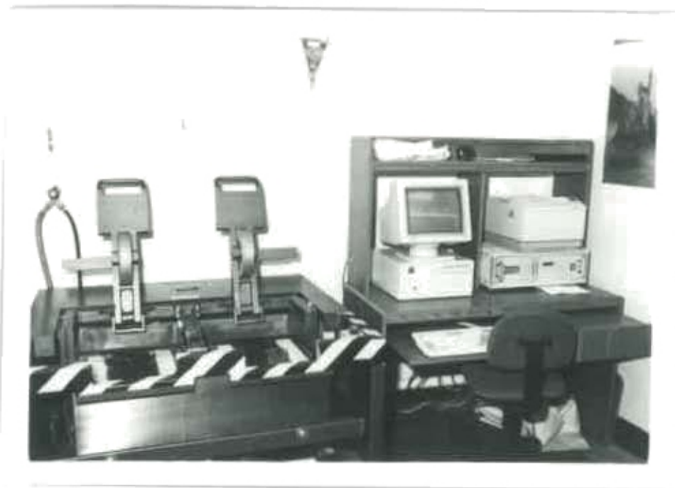
Fig. 1. The Hamburg Wheel-Tracking Device.
