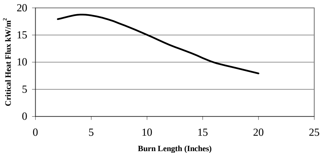
FIGURE 21. INVERSE RELATIONSHIP BETWEEN FLAME PROPAGATION AND CRITICAL RADIANT FLUX
