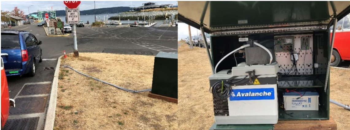
Figure 3 - (left) Sampled Catchbasin and Piping; (right) Sampling Equipment (Autosampler, Datalogger, Battery, etc)
